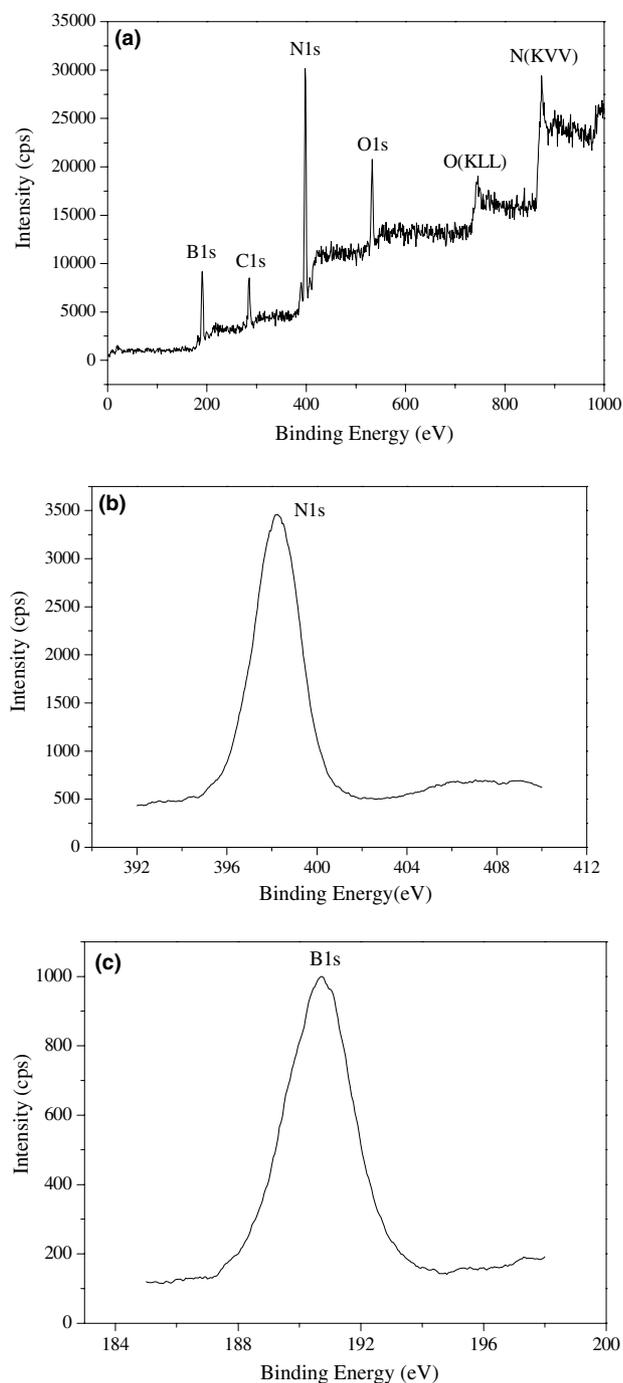
Fig. 3. XPS spectra of the h-BN sample prepared at 600 °C, 12 h: (a) survey spectrum; (b) N1s region; (c) B1s region.
