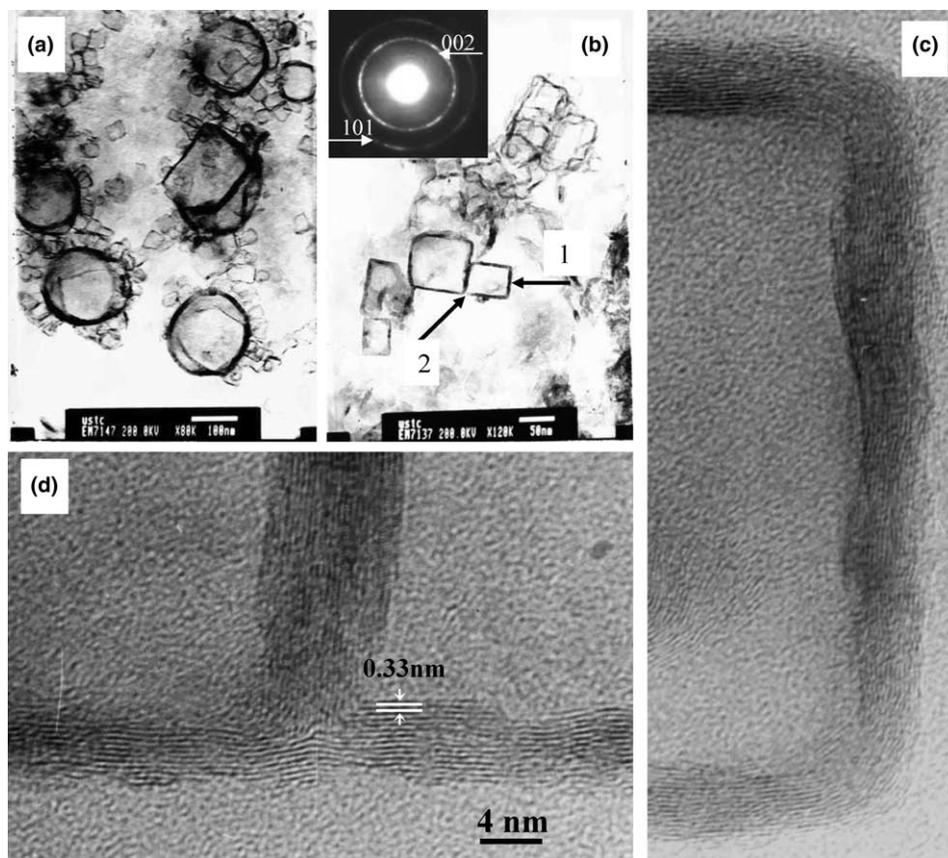
Fig. 2. TEM and HRTEM images of sample C. (a) TEM images of nanocages of sample C: prepared at 600 °C, 12 h. (b) High-resolution TEM images of sample C. Inset: the corresponding SAED pattern of the h-BN powder. (c) HRTEM images of the box-like nanocage (marked by arrow 1 in Fig. 2b). (d) HRTEM images of two connected cages sharing the same wall (marked by arrow 2 in Fig. 2b).
