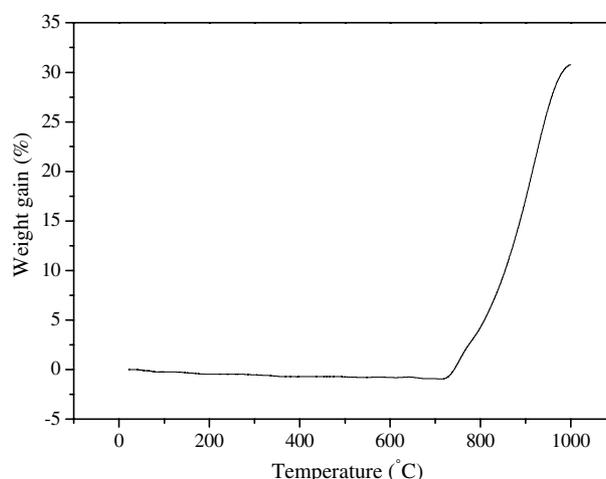
Fig. 4. TGA curve of the h-BN sample prepared at 600 °C, 12 h.
