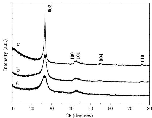
Fig. 1. XRD patterns of the prepared samples. (a) Sample A: prepared at 400 °C, 12 h; (b) Sample B: prepared at 500 °C, 12 h; (c) Sample C: prepared at 600 °C, 12 h.
