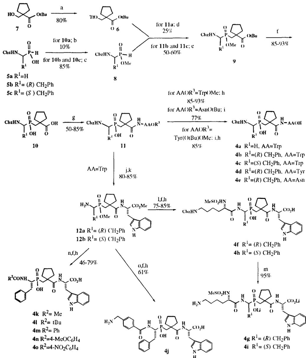
Reagents: (a) 1.5 equiv. Tf<sub>2</sub>O, 7 eq. pyridine, CH<sub>2</sub>Cl<sub>2</sub>, -78°-0°C; (b) DEC, DMAP, MeOH; (c) CH<sub>2</sub>N<sub>2</sub>, EtOAc, MeOH; (d) NaH, THF, **6**, 0°C-rt; (e) LDA, THF, -78°C then **6** -78°C to rt; (f) HCl, 1,4-dioxane; (g) L-AAOMe.HCl.
