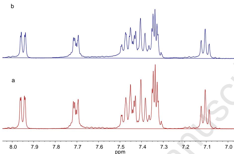
**Fig. 5.** Partial  $^1\text{H}$  NMR spectra of **2** with (a) and without (b) addition of  $\text{LaCl}_3 \cdot 7\text{H}_2\text{O}$  (solvent:  $\text{DMSO-d}_6$ ).
