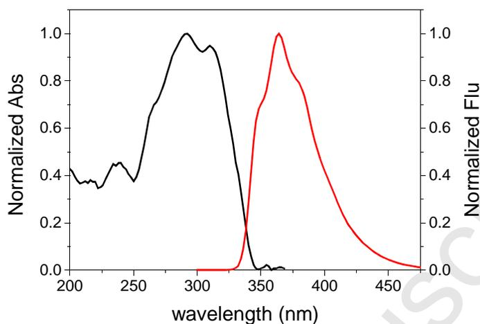
**Fig. 4.** Absorption and fluorescence of **2** in DMSO solution (50  $\mu$ M, irradiation wavelength:  $\lambda_{\text{ex}} = 290$  nm).
