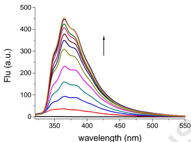
**Fig. 3.** Fluorescence changes of **1** (50 $\mu$ M, in DMSO) with UV light irradiation (irradiation wavelength:  $\lambda = 254$  nm, irradiation periods: 0, 2, 4, 6, 8, 10, 12, 14, 16, 18, 20, 22 min, excitation wavelength:  $\lambda_{\text{ex}} = 290$  nm).
