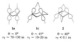
According to the Salem rule,<sup>4</sup> optimal spin-orbit coupling, i.e., fast intersystem crossing and consequently short triplet lifetimes, should prevail when the two interacting radical orbitals are oriented at each other with a 90° interorbital angle. The total angular momentum is then conserved, since the change in the spin angular momentum is exactly offset by the change in orbital momentum during the intersystem crossing process.
