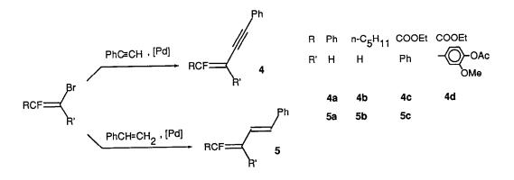
Reaction conditions : alkene or alkyne 1-2 equiv.,  $Pd(OAc)_2 0.02$  equiv.,  $PPh_3 0.04$  equiv., triethylamine, reflux, 3 h.
