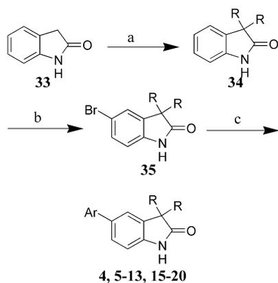
**Scheme 1.** Reagents and conditions: (a) *n*-BuLi, TMEDA, THF  $-78^{\circ}\text{C}$ , then R-I; (b)  $\text{Br}_2$ , NaOAc, AcOH, rt; (c)  $\text{Pd}(\text{Ph}_3\text{P})_4$ ,  $\text{ArB}(\text{OH})_2$ ,  $\text{Na}_2\text{CO}_3$ , DME– $\text{H}_2\text{O}$ ,  $90^{\circ}\text{C}$ .
