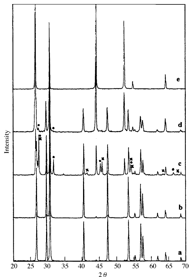
Fig. 4 X-Ray powder patterns of fresh (a) \text{Nd}_2\text{O}_3 (b)–(d) 25, 50, 80 mol.% \text{SrF}_2 - \text{Nd}_2\text{O}_3 , (e) \text{SrF}_2 . (x) Rhombohedral \text{NdOF} , (o) tetragonal \text{NdOF} .
