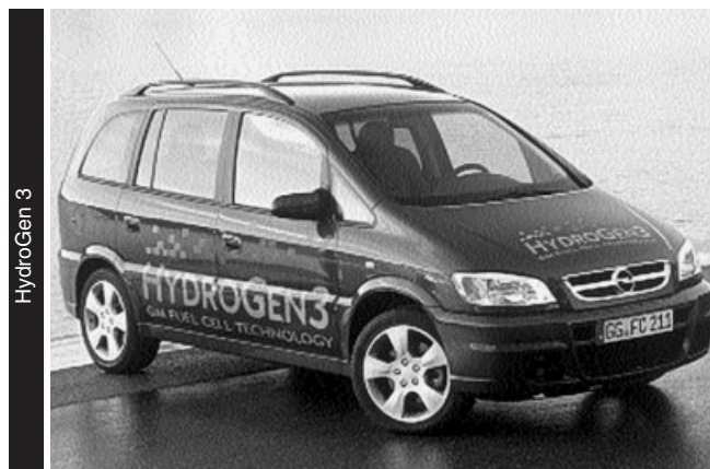
Fig. 1 The HydroGen3 based on the Opel Zafira series model.
