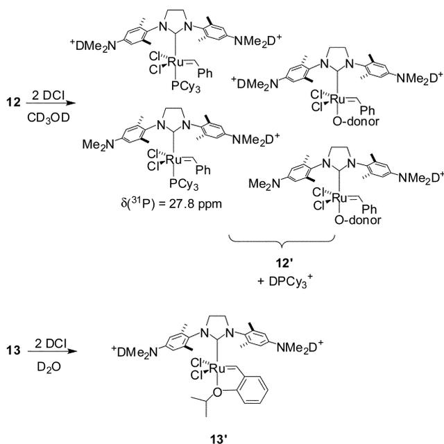
**Scheme 3** Reaction of catalysts **12** and **13** with DCl (2 equiv.).
