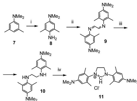
**Scheme 2** Preparation of H<sub>2</sub>ITap-HCl **11**: (i) (1) NaNO<sub>2</sub>/conc. HCl<sub>aq</sub>, 60 min, –5 °C, (2) Sn/HCl, 70 °C (45%); (ii) (CHO)<sub>2</sub>/MeOH [HCl], 24 h, RT (85%); (iii) NaBH<sub>4</sub>/H<sub>3</sub>BO<sub>3</sub>/thf, 60 min, 30 °C (88%); (iv) HC(OEt)<sub>3</sub>/NH<sub>4</sub>Cl, 12 h, 130 °C (87%).
