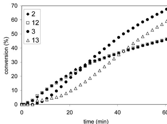
**Fig. 4** RCM of DEDAM with catalysts **2**, **3**, **12**, **13** ([Ru] = 0.5 mM, 0.5% catalyst loading).
