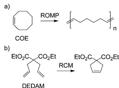
**Scheme 4** Olefin metathesis reactions with catalysts **2**, **3**, **12**, **13** in benzene (20 °C). (a) ROMP of COE ([Ru] = 0.5 mM, 0.5% loading); (b) RCM of DEDAM ([Ru] = 1.0 mM, 1.0% loading).
