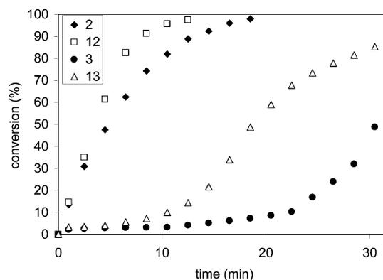
**Fig. 3** ROMP of COE with catalysts **2**, **3**, **12**, **13** ([Ru] = 0.5 mM, 0.5% catalyst loading).
