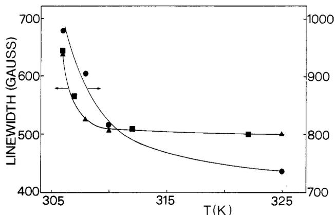
Figure 5. ESR line width as function of temperature: (●) iridium containing sample, (▲) rhodium containing sample, (■) pure chromia.
