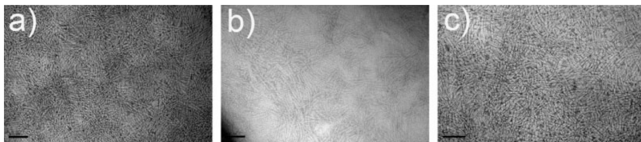
FIGURE 6 TEM images (negatively stained with uranyl acetate) of sample cast from aqueous solution of (a) 1 , (b) 2 , and (c) 3 (scale bar = 100 nm).
