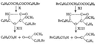
With the cyclic character of the ethers established in this manner, the cyclic structure of substances related in origin and similar in properties can be accepted with confidence. Thus the acetate which is formed by the action of acetic anhydride on the triketone must be a furanone derivative because it passes into the ethers when it is dissolved in boiling alcohols.
