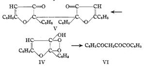
In accordance with the mechanism which has been established in more favorable cases in which all the intermediates were isolated, the triketone, doubtless, is the final product in a series of transformations which can be represented as follows
