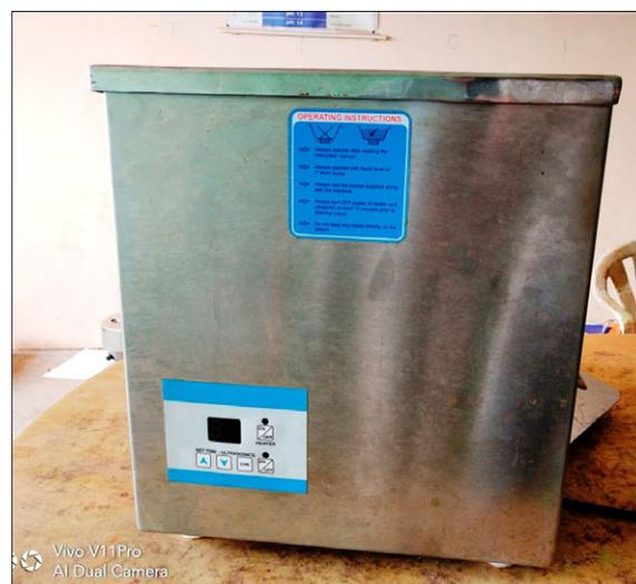
**FIGURE 1** Ultrasonication (frequency of 50 Hz and power of 250 V AC, 5.5 L and temperature 70°C)
