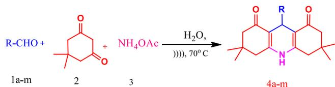
**SCHEME 1** General reaction of 3,3,6,6-tetramethyl-9-substituted phenyl-3,4,6,7,9,10-hexahydroacridine-1,8(2H,5H)-dione
