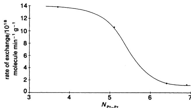
Fig. 4 Dependence of rate of the exchange on  $N_{\text{Pt-Pt}}$  in mazzites.  $P_{\text{D}_2} = P_{\text{CH}_4} = 100$  mbar.
