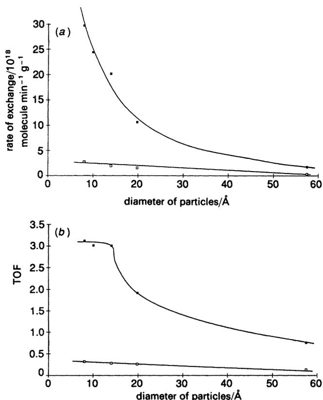
Fig. 3 Rate of deuterium exchange in methane (a) and turnover frequency (b) on Pt/Al<sub>2</sub>O<sub>3</sub> with different particle sizes.  $P_{\text{D}_2} = P_{\text{CH}_4} = 100$  mbar;  $T/\text{K}$ : □, 460; ■, 500.
