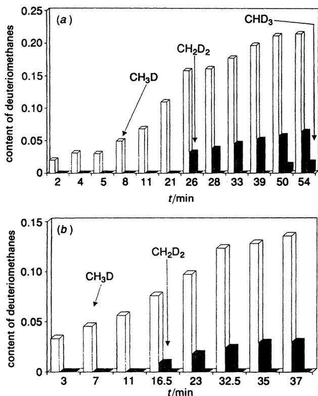
Fig. 2 Distribution of products for the exchange of methane on supported catalysts: (a) 5Pt/Al<sub>2</sub>O<sub>3</sub>,  $T = 500$  K,  $P_{\text{CH}_4} = P_{\text{D}_2} = 100$  mbar; (b) 3PtMaz,  $T = 460$  K,  $P_{\text{CH}_4} = P_{\text{D}_2} = 100$  mbar
