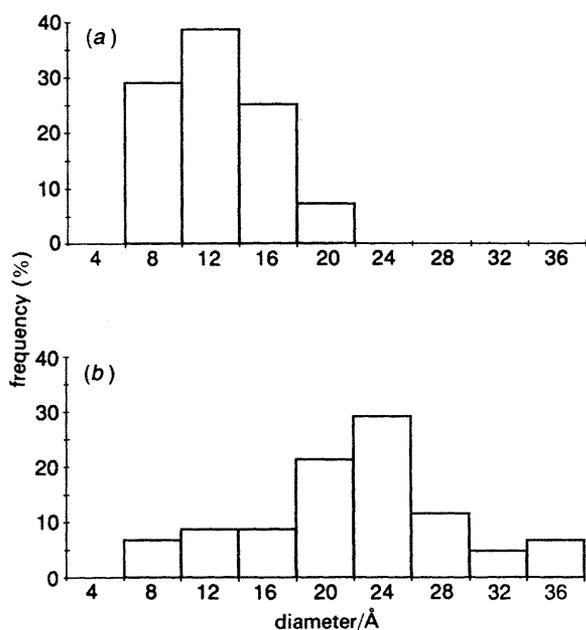
**Fig. 1** Histograms of particle size for various Pt/Maz zeolites: (a) 1PtMaz,  $d_{av} = 12.4$  Å; (b) 4PtMaz,  $d_{av} = 22.3$  Å
