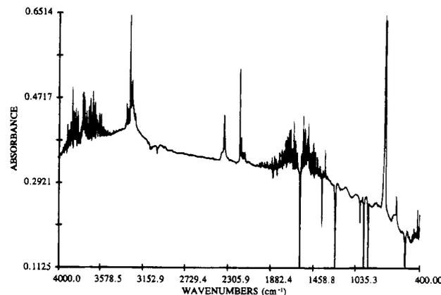
**Figure 4.** FTIR difference spectrum after 360 min Hg lamp photolysis of C<sub>2</sub>H<sub>3</sub>I/Ar (1/10 000). The fine structure near  $3700$  and  $1600 \text{ cm}^{-1}$  is due to water vapor.
