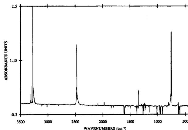
**Figure 1.** FTIR difference spectrum after 450 min Hg lamp photolysis of  $\text{C}_2\text{H}_3\text{Br/Kr}$  (1/100).
