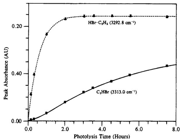
**Figure 2.** Growth behavior of HBr-C<sub>2</sub>H<sub>2</sub> complexes and C<sub>2</sub>HBr as a function of Hg lamp photolysis time (C<sub>2</sub>H<sub>3</sub>Br/Kr = 1/100).
