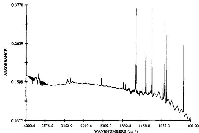
**Figure 3.** FTIR spectrum of vinyl iodide/Ar (1:10 000). The negative going fine structure near  $3700$  and  $1600 \text{ cm}^{-1}$  is due to interference from gas phase water.
