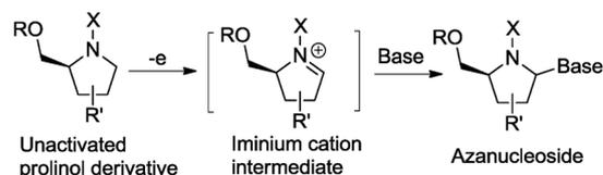
Fig. 1 Schematic view of an electrochemically direct transformation reaction of non-activated prolinol derivatives for the synthesis of azanucleosides.
