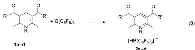
Formation of the borohydride anion was confirmed by its characteristic doublet at  $-25 \text{ ppm}$  in the  $^{11}\text{B}$  NMR spectra. The reactions initiate rapidly at temperatures below  $-40^\circ\text{C}$ , with no further conversion being observed after 30 min at  $-20^\circ\text{C}$ .<sup>[40]</sup>
