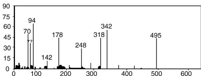
Fig. 2. Electron impact mass spectrum of the ligand (L).
