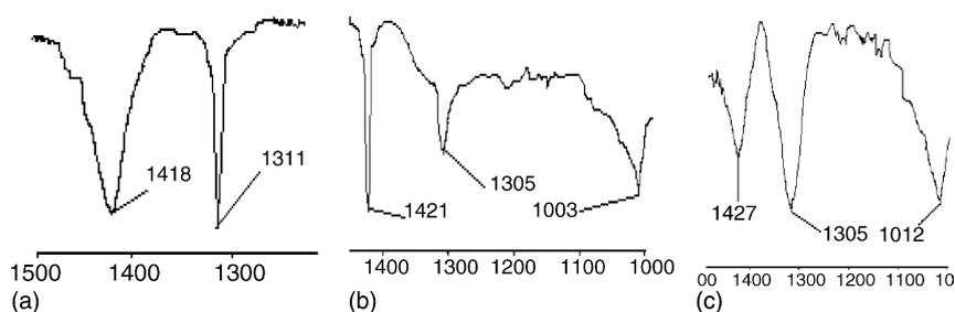
Fig. 3. IR spectral bands of anions (a)  $[\text{Co}(\text{L})(\text{NO}_3)_2]$ ; (b)  $[\text{Ni}(\text{L})(\text{NO}_3)_2]$ ; (c)  $[\text{Cu}(\text{L})(\text{NO}_3)_2]$ .
