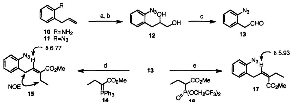
Scheme 1. Reagents and conditions: (a) HCl, NaNO<sub>2</sub>, H<sub>2</sub>O, 0 °C, 15 min, then NaN<sub>3</sub>, 0 °C, 30 min, 83%; (b) OsO<sub>4</sub>, *N*-methylmorpholine *N*-oxide (NMO), acetone-H<sub>2</sub>O (1:1), rt, 17 h, 89%;<sup>12</sup> (c) NaIO<sub>4</sub>, THF-H<sub>2</sub>O (1:1), rt, 4.5 h, 70%; (d) **14**, CH<sub>2</sub>Cl<sub>2</sub>, rt, 30 h, 80% (*E*:*Z*=32:1); (e) **16**, KN(TMS)<sub>2</sub>, 5 equiv of 18-crown-6, THF, -78 °C→rt, 4 h, 50% (*E*:*Z*=1:8).
