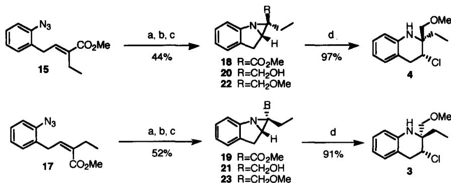
Scheme 2. Reagents and conditions: (a)  $h\nu$ , toluene, rt; (b) LiAlH<sub>4</sub>, THF, 0 °C; (c) KH, THF, 0 °C, 30 min, then 5 equiv of MeI, -15 °C; (d) 15 equiv of Et<sub>4</sub>NCl, TFA, CH<sub>2</sub>Cl<sub>2</sub>, -15 °C, 20 min.
