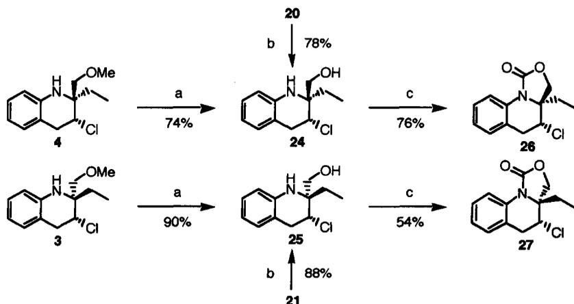
Scheme 3. Reagents and conditions: (a)  $\text{AlCl}_3$ , *n*-PrSH,  $\text{CH}_2\text{Cl}_2$ , rt; (b) 15–20 equiv of  $\text{Et}_4\text{NCl}$ , TFA,  $\text{CH}_2\text{Cl}_2$ ,  $-15$  °C, 20 min; (c) 10 equiv of  $\text{Im}_2\text{CO}$ , toluene, 60–100 °C.
