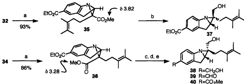
Scheme 5. Reagents and conditions: (a) *hν*, toluene, rt, 3 h; (b) 4 equiv of LiAlH(*O*-*t*-Bu)<sub>3</sub>, THF, rt, 14 h, 93%; (c) LiAlH<sub>4</sub>, THF, 0 °C, 3 h, 100%; (d) MnO<sub>2</sub>, acetone, rt, 46 h; (e) KCN, MnO<sub>2</sub>, MeOH, rt, 3.5 h, 82% (2 steps).
