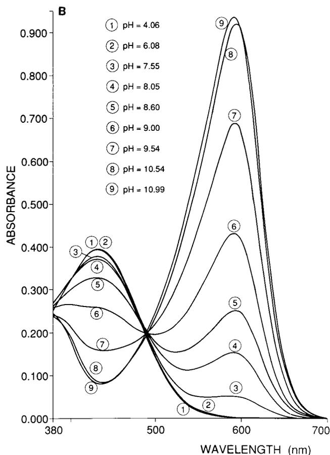
FIG. 5B. Absorption spectra of XB in solution ( $C = 10^{-5}$  M) in the basic range.
