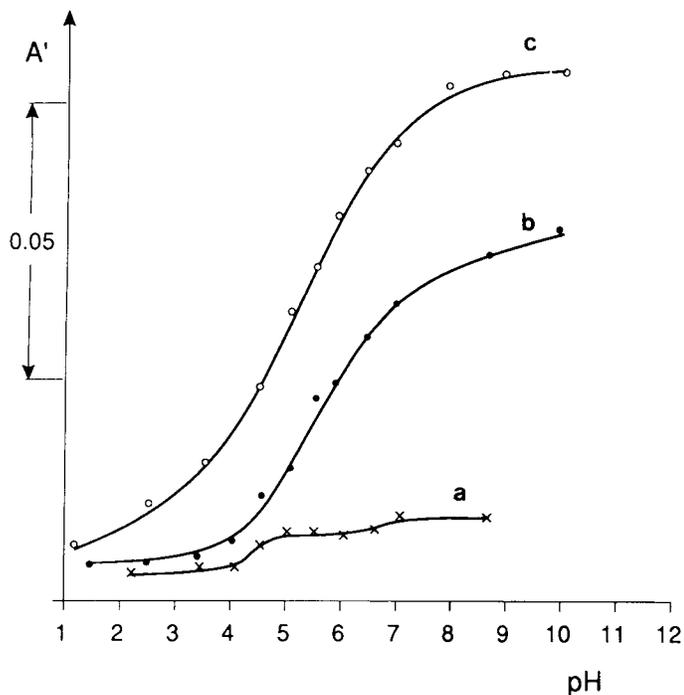
FIG. 2.  $A'$  values measured at the absorption peak vs. pH for BPB for the three methods followed: (a) first method; (b) second method; (c) third method.
