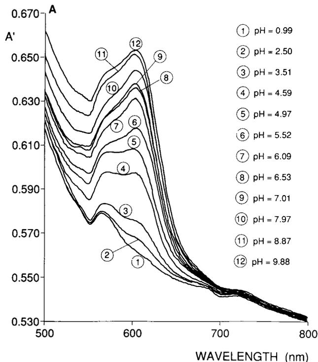
FIG. 1A. Reflectance spectra of BPB immobilized on quartz powder for different pH values following the third immobilization method.
