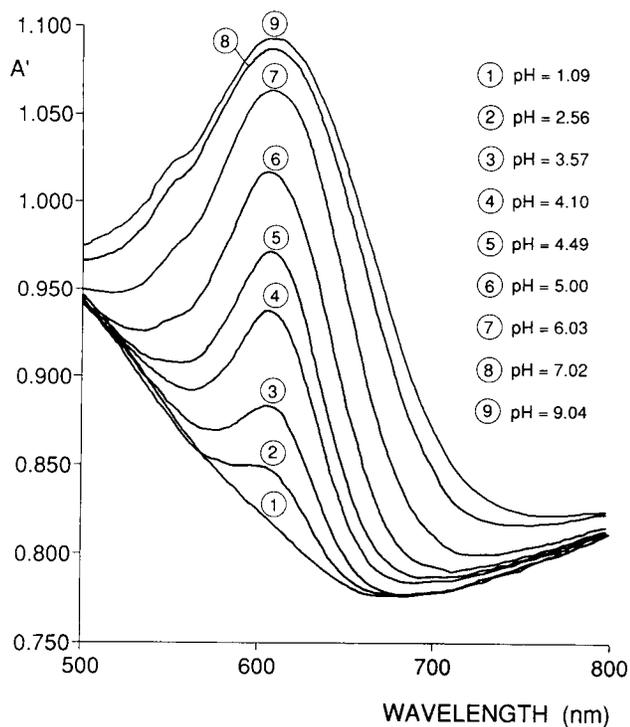
FIG. 6. Reflectance spectra of BPB immobilized on CPG for different pH values.
