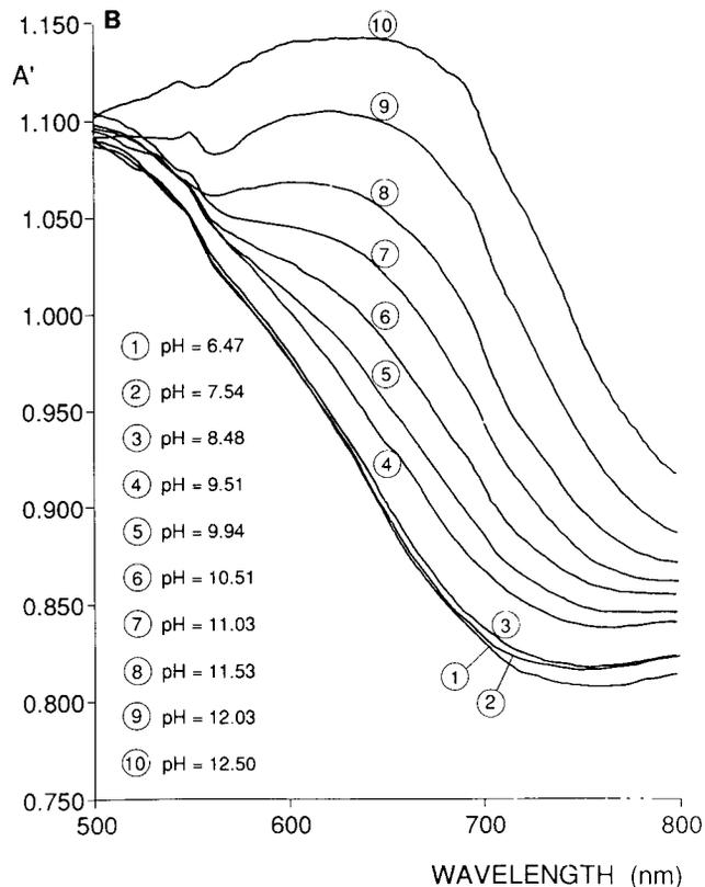
FIG. 9B. Reflectance spectra of XB immobilized on CPG for different pH values in the basic range.
