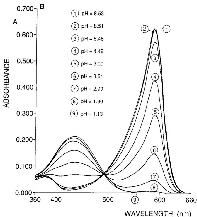
FIG. 1B. Absorption spectra of BPB in solution ( $C = 10^{-5}$  M) for different pH values.
