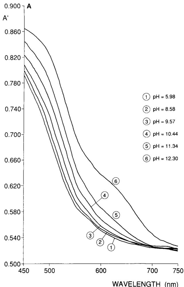
FIG. 5A. Reflectance spectra of XB immobilized on quartz powder in the basic range following the third immobilization method.
