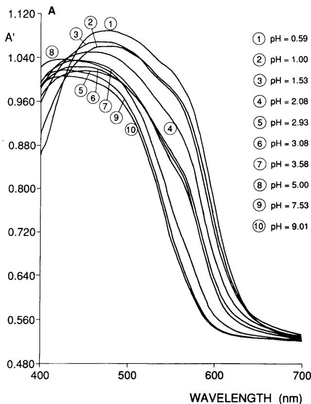
FIG. 3A. Spectra of DMA immobilized on quartz powder for different pH values according to the third immobilization method.
