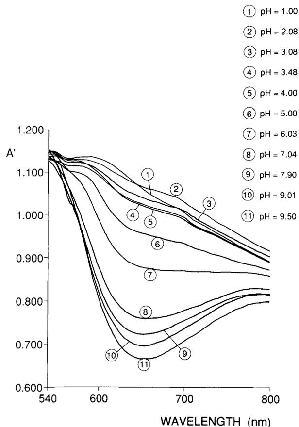
FIG. 8. Reflectance spectra of DMA immobilized on CPG for different pH values.
