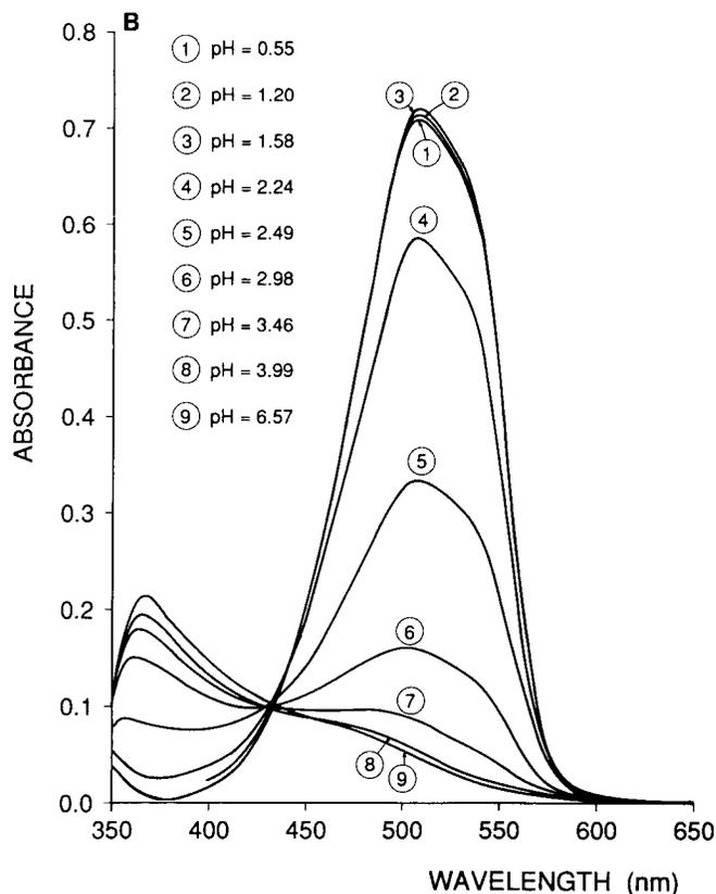
FIG. 3B. Absorption spectra of FIDMA in solution ( $C = 10^{-5} \text{ M}$ ) for different pH values.
