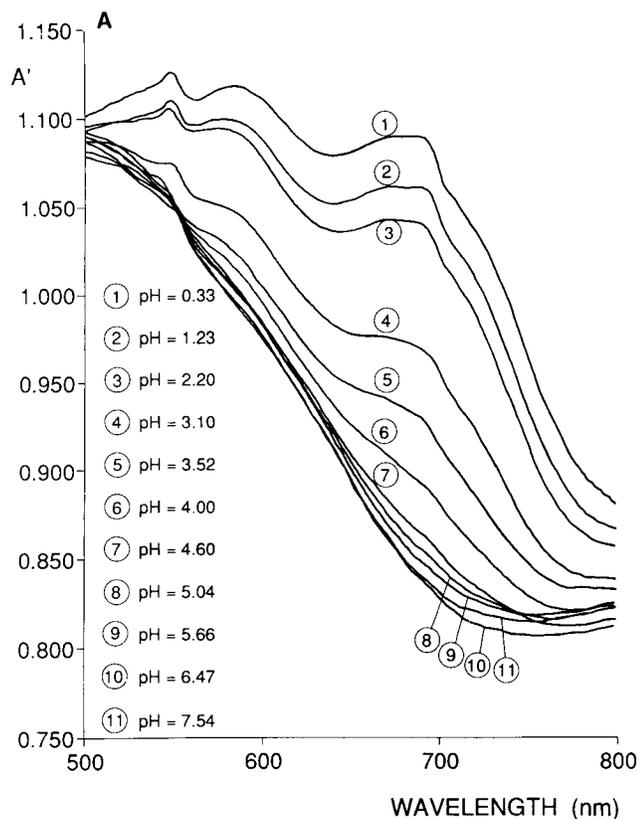
FIG. 9A. Reflectance spectra of XB immobilized on CPG for different pH values in the acidic range.
