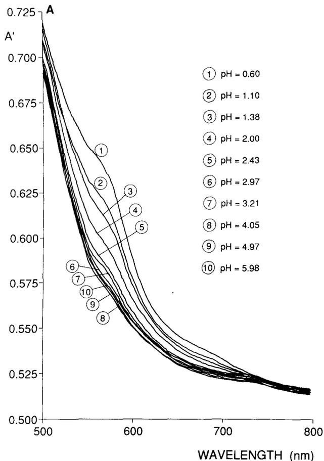
FIG. 4A. Reflectance spectra of XB immobilized on quartz powder in the acidic range following the third immobilization method.
