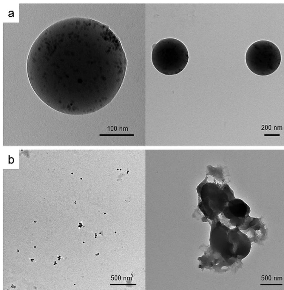
**FIGURE 5** Representative TEM images of nanoparticles; either unirradiated (a) or irradiated for 5 min with 350 nm UV light (b) after 1 day incubation at 37 °C in dilute triethylamine/ water solution (pH 8.0).
