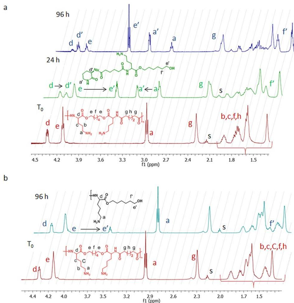
**FIGURE 4** <sup>1</sup>H NMR spectra of deprotected polymer **1-Boc** (a) and **2-Boc** (b) in deuterium phosphate buffer (0.2 M) at pH 7.4, as a function of incubation time (37 °C).
