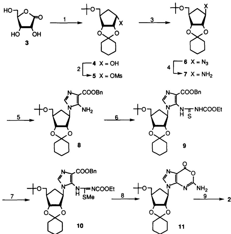
**Scheme 1 Reagents and Conditions:** 1) 6 steps. See ref.5; 2) MsCl, Et<sub>3</sub>N, CH<sub>2</sub>Cl<sub>2</sub>, 0 °C, 1 h; 3) NaN<sub>3</sub>, DMF, 120 °C, 18 h; 4) LiAlH<sub>4</sub>, THF, 0 °C, 2.5 h; 5) EtO-CH=N-CH(CN)COOBn, EtOH, reflux, 30 min; 6) EtOCONCS, CH<sub>3</sub>CN, reflux, 2 h; 7) 0.1 N-NaOH, MeI, rt, 2 h; 8) 5N-KOH, MeOH, reflux, 30 min; 9) CF<sub>3</sub>COOH-H<sub>2</sub>O (2:1), 50 °C, 3 h.
