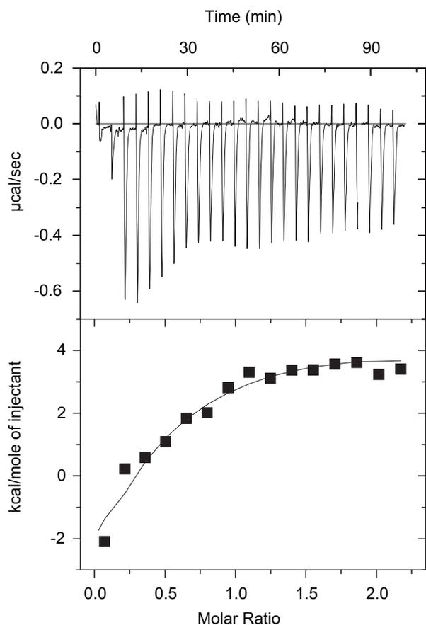
Fig. 11. Isothermal titration of  $\text{Cu}(\text{OAc})_2$  solution into  $\text{pol1}$  in methanol at 300 K.
