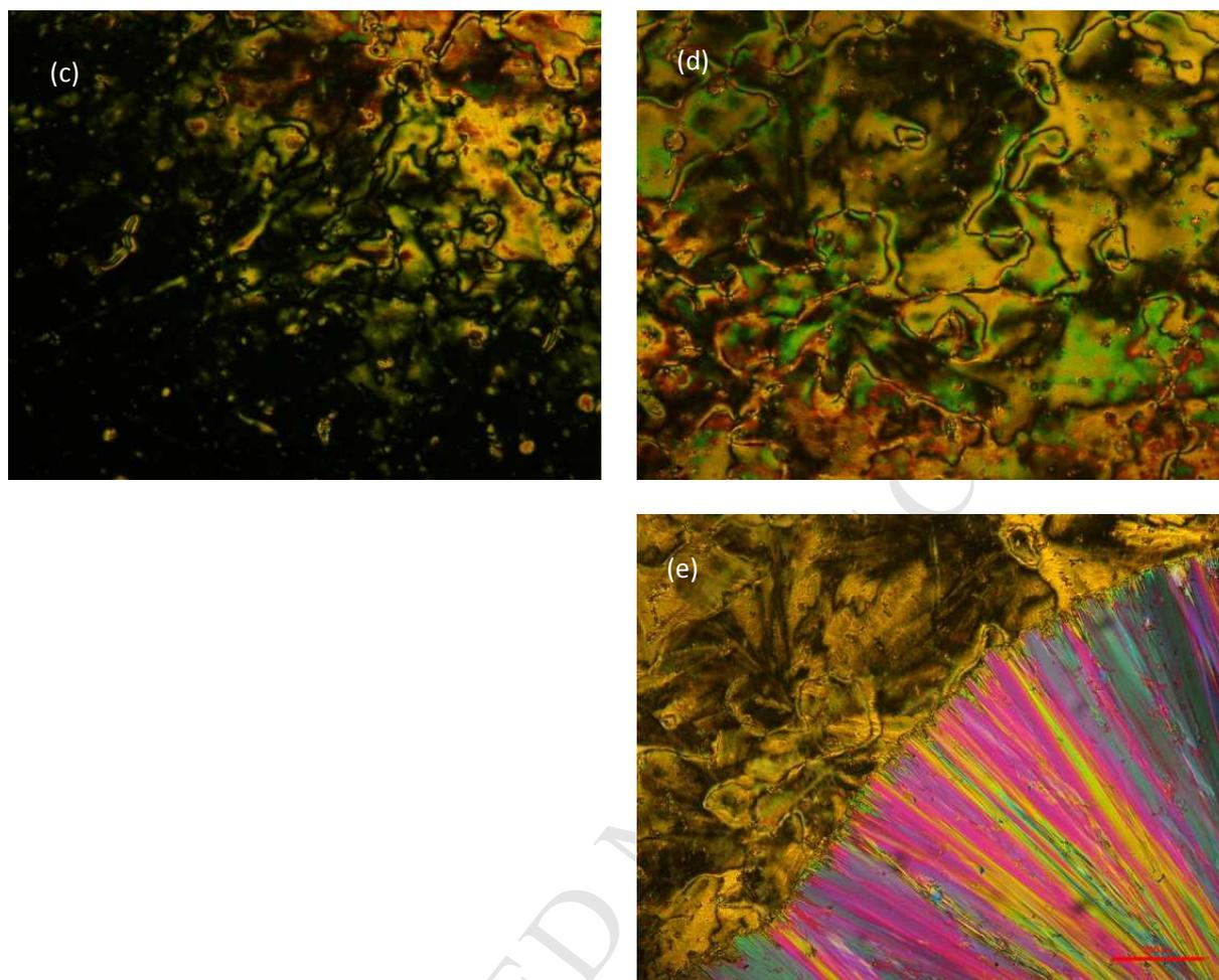
**Fig 4.** Polarising optical microscopic textures of the compound (**5b**). (a) Growth of the schlieren texture from isotropic liquid at 127.7 °C; (b) homeotropic texture at 127.6 °C; (c) appearance of thread like texture from homeotropic region at 127.5 °C; (d) thread texture of the nematic phase at 127.4 °C; (e) Co-existence of N-Cr transition at 54.9 °C.
