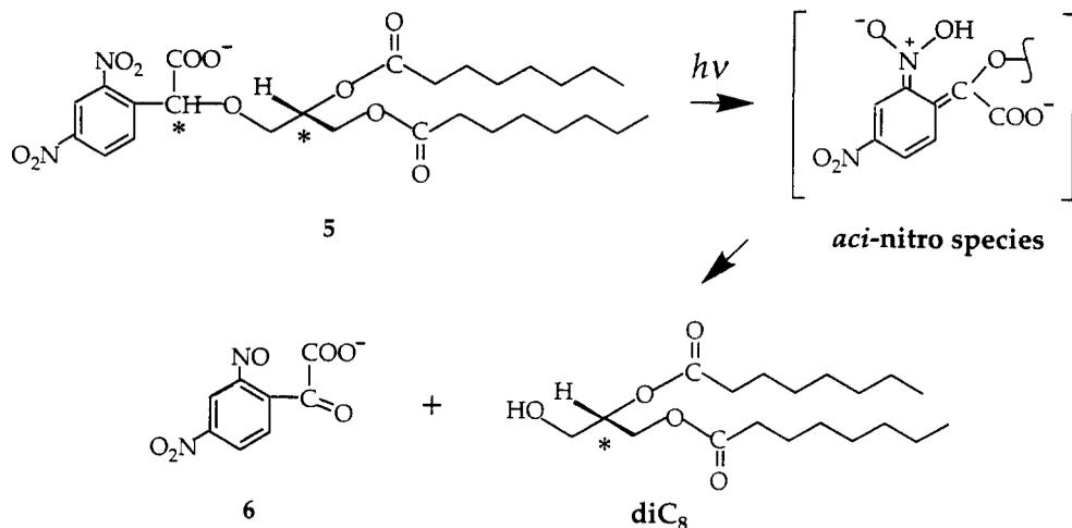
Scheme 2. Proposed photolysis reaction for  $\alpha$ -carboxyl caged  $diC_8$ .
