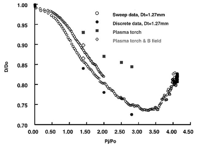
Fig. 12 Drag data of plasma injection vs  $P_j/P_0$ .
