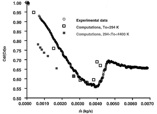
Fig. 7 Drag distribution vs injecting mass flow rate.
