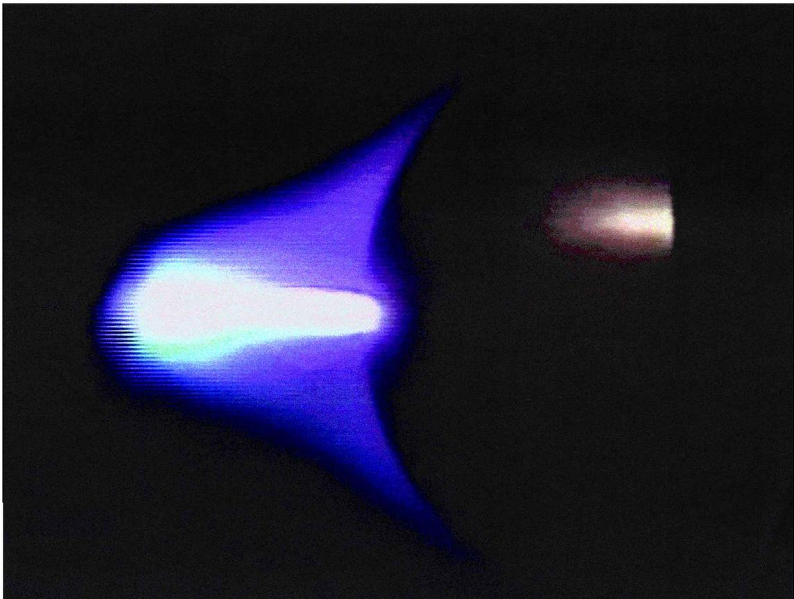
Fig. 9 Plasma counterflow jet and shock interaction.
