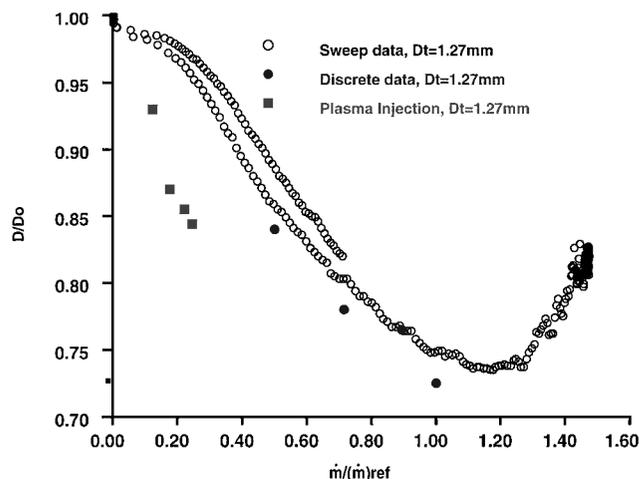
Fig. 13 Drag data of plasma injection vs  $m/(m)_{ref}$ .
