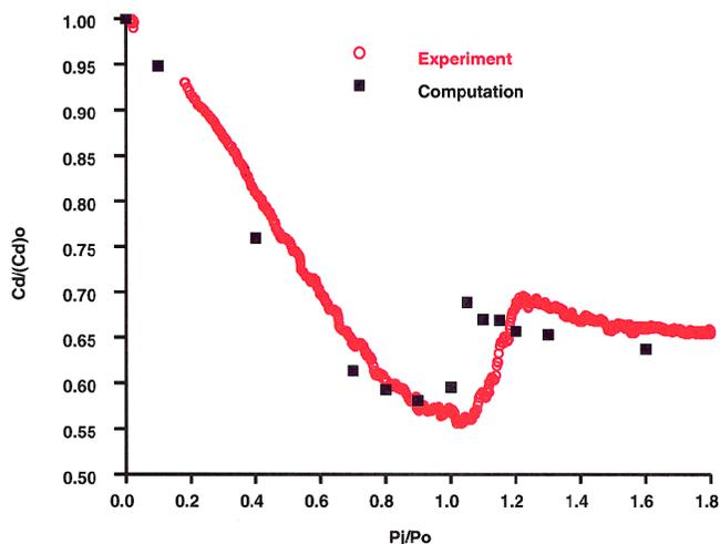
Fig. 3 Comparison of computed and measured drag.
