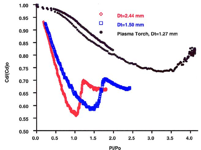
Fig. 2 Drag data of counterflow jet interaction.
