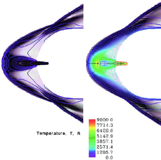
Fig. 8 Flowfield structures at different stagnation temperatures.
