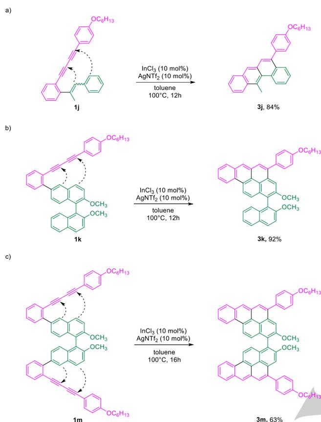
**Scheme 2.** Domino benzannulation reaction of alkynes in (a) stilbene derivative, (b-c) dimethoxy-1,1'-binaphthalene derivatives.
