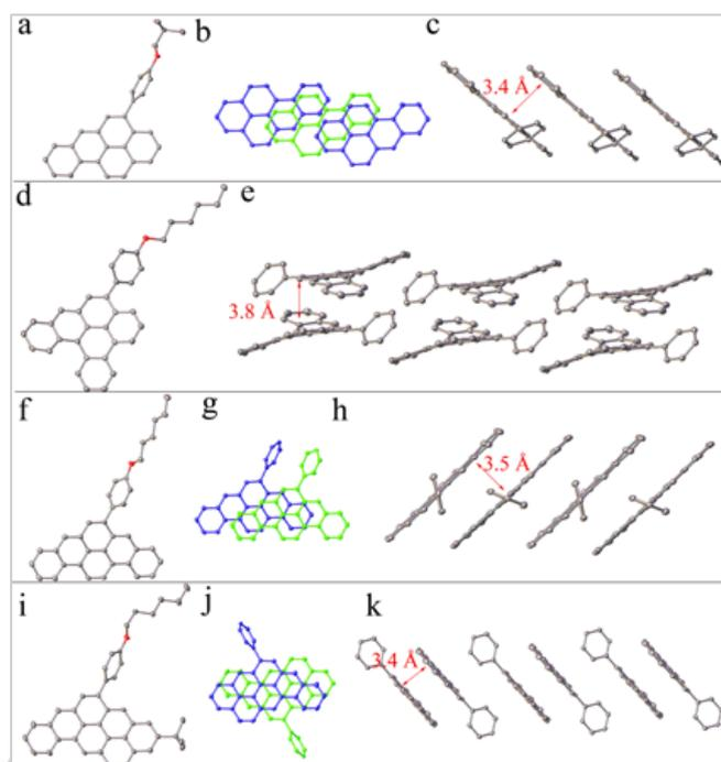
**Figure 2.** X-ray structures (ellipsoids at 50% probability, hydrogens removed for clarity) and packing structures (hydrogens and side chains removed for clarity) of (a-c) **3a**, (d-e) **3d**, (f-h) **3e**, and (i-k) **3f**.
