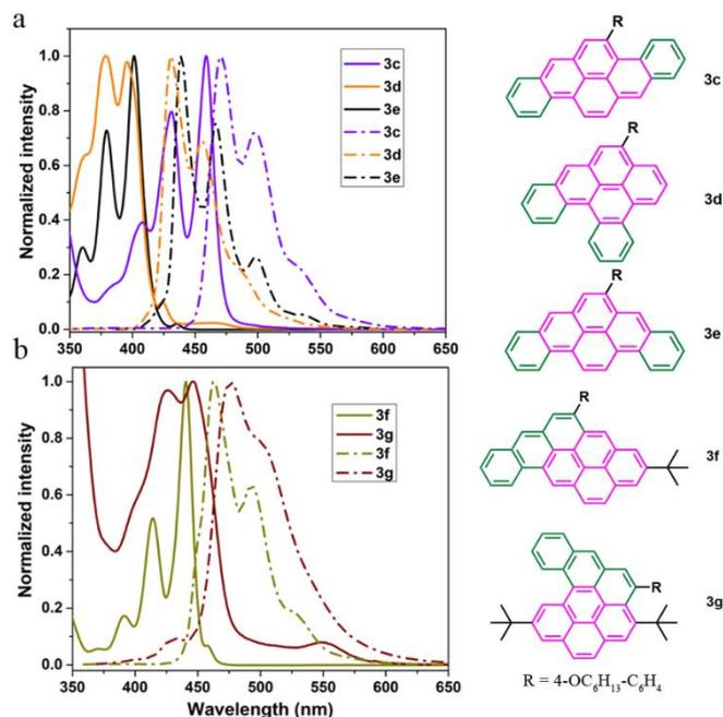
**Figure 3.** The UV-Vis absorption (solid line) and emission (dash-dot line) spectra of selected (a) dibenzochrysenes compounds **3c**, **3d**, **3e** and (b) compounds **3f** and **3g** in toluene at 298 K.
