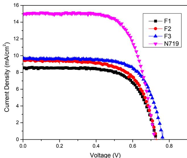
Fig. 6. Current - potential ( $J$ - $V$ ) curve for the DSSCs based on **F1**, **F2** and **F3**.
