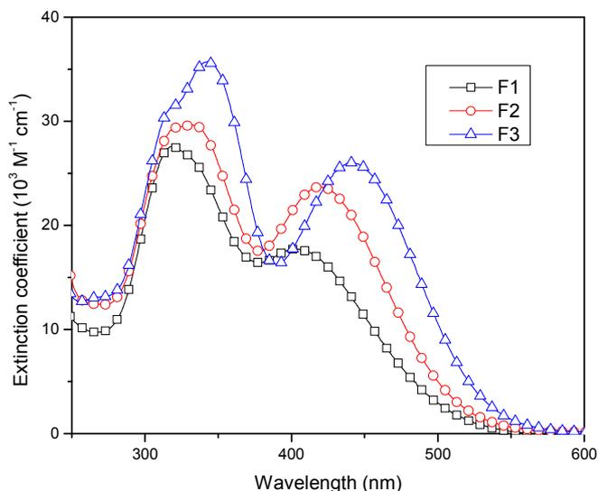
Fig. 2. Absorption spectra of **F1**, **F2**, and **F3** in  $\text{CH}_2\text{Cl}_2$  at ambient temperature.
