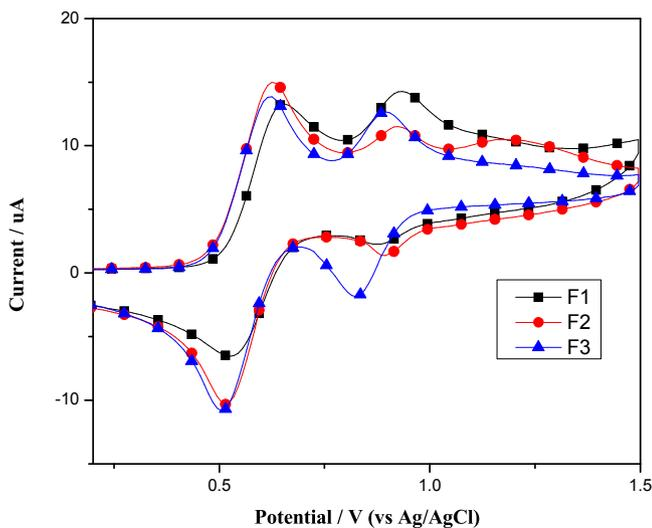
Fig. 4. Cyclic voltammogram of **F1**, **F2**, and **F3** in CH<sub>2</sub>Cl<sub>2</sub>.
