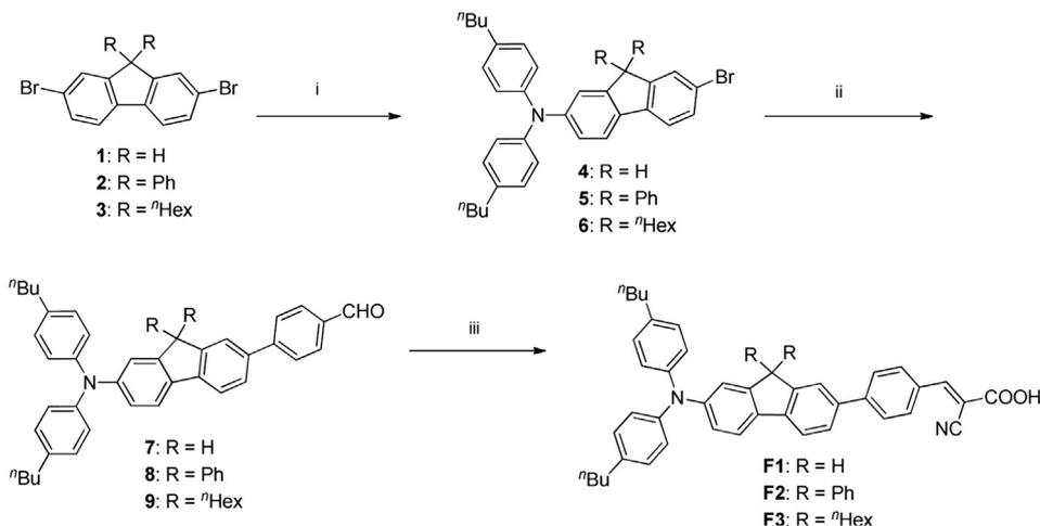
Scheme 1. The synthetic routes for **F1**, **F2** and **F3** dyes: i) bis(4-butylphenyl)amine,  $\text{Pd}(\text{dba})_2$ , dppf,  $t\text{BuONa}$ , toluene, 110 °C; ii) (4-formylphenyl)boronic acid,  $\text{Pd}(\text{PPh}_3)_4$ ,  $\text{K}_2\text{CO}_3$ , THF, refluxed; iii) cyanoacetic acid,  $\text{NH}_4\text{OAc}$ , glacial  $\text{CH}_3\text{COOH}$ , refluxed.
