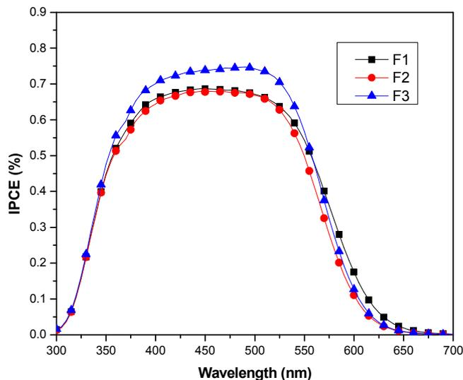
Fig. 5. IPCE spectra for DSSCs based on the as-synthesized dyes.
