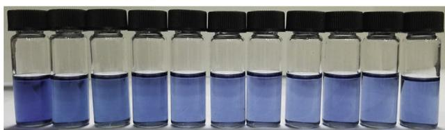
Fig. 7. Photographs showing the colorimetric changes for **3a-c** in DMF/water ( $v:v = 8:2$ ) solution upon addition of 0.0–2.0 eq of  $\text{Hg}^{2+}$  (left to right). The concentrations of **3a-c** are all closed to  $1.0 \times 10^{-5}$  mol/L.
