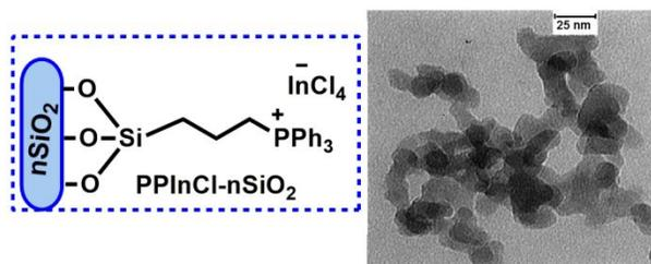
**Figure 1.** The schematic structure of PPIInCl-nSiO<sub>2</sub> along with its TEM image
