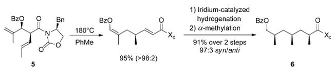
**Scheme 2.** Stereoselective synthesis of trideoxypropionates **6**.<sup>[10]</sup>
