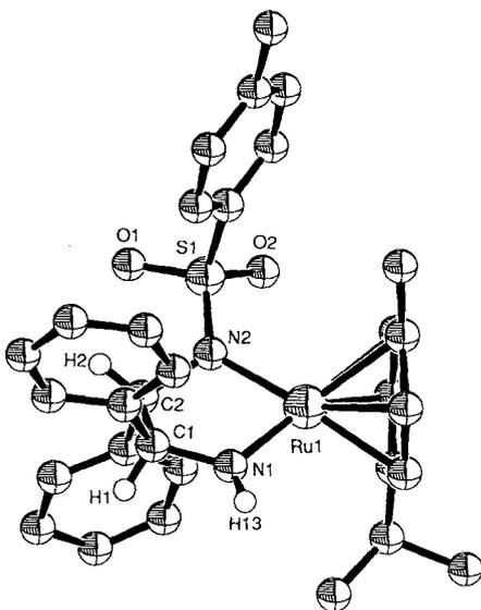
Figure 2. Molecular structure of **2** in the crystal. All hydrogen atoms except for the proton of the amide ligand and those at the carbon atoms in the chelate backbone have been omitted for the sake of clarity. Selected distances [Å] and angles [°]: Ru–N1 1.897(6), Ru–N2 2.065(6), N1–H13 0.88(6); N1–Ru–N2 78.9(2), Ru–N1–C1 121.2(5), Ru–N2–C2 114.9(4).
