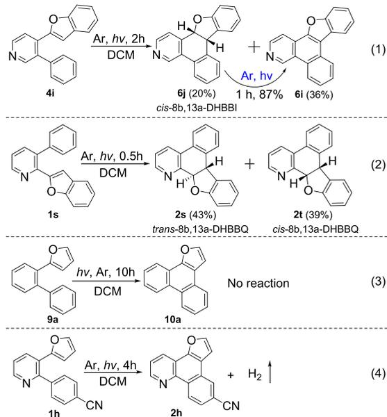
**9a** under the same conditions (500 W high-pressure mercury lamp) failed to provide dehydrogenative annulation to **10a** (Scheme 5, eq 3). Thus, it is easy to conclude that the presence of nitrogen in the pyridine and pyrimidine ring is critical.
