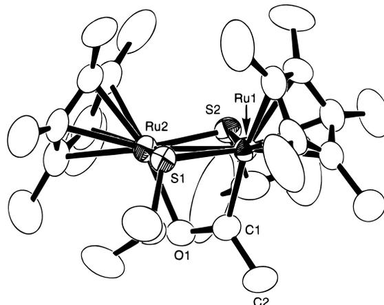
Figure 2. ORTEP drawing for the cationic part of **5**. Hydrogen atoms are omitted for clarity.
