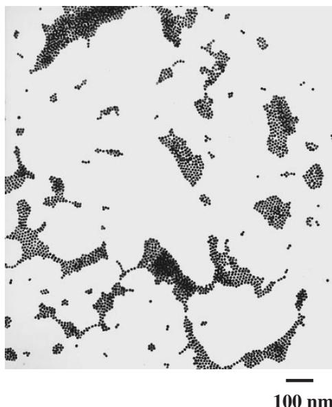
Fig. 2. TEM images of Au/HS(CH<sub>2</sub>)<sub>10</sub>COOH colloids at pH 6.
