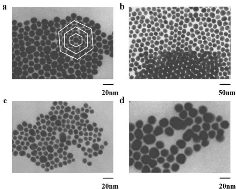
Fig. 3. TEM images of (a) Au/HS(CH<sub>2</sub>)<sub>10</sub>COOH, (b) Au/EtSS(CH<sub>2</sub>)<sub>10</sub>COOH, (c) Au/HS(CH<sub>2</sub>)<sub>15</sub>COOH, and (d) Au/EtSS(CH<sub>2</sub>)<sub>15</sub>COOH colloids. All samples were controlled at pH 6.
