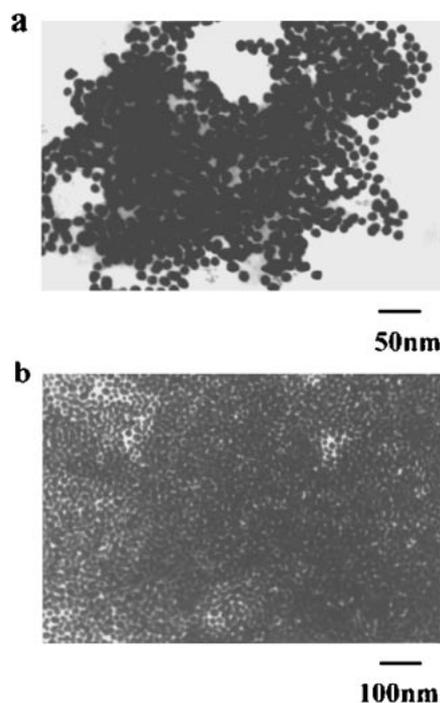
Fig. 5. TEM images of (a) and (b) show the assemblies of the colloidal Au/HS( $\text{CH}_2$ ) $_{10}$ COOH at pH 11 and 3, respectively.
