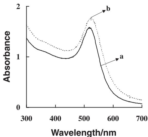
Fig. 1. UV-vis absorption spectra of (a) Au colloidal solution and (b) Au/HS(CH<sub>2</sub>)<sub>10</sub>COOH colloids.
