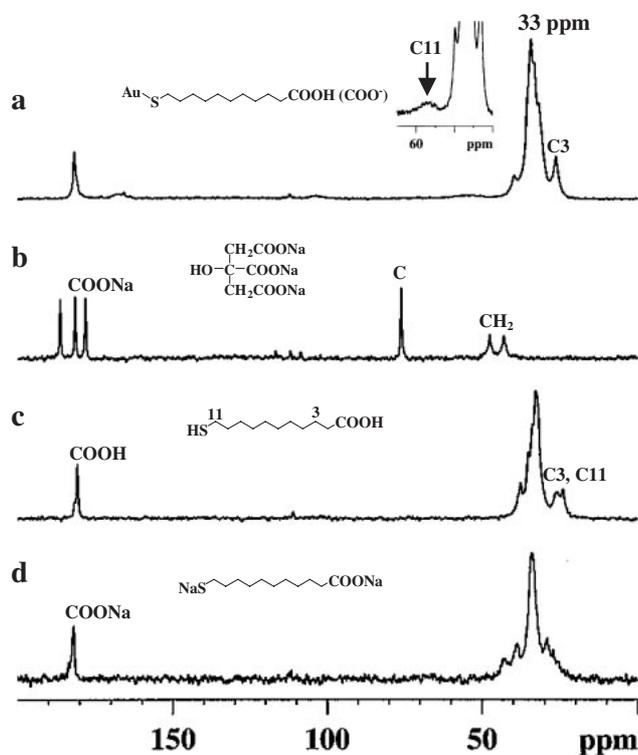
Fig. 4. Solid-state  $^{13}\text{C}$ NMR spectrum of (a) Au/HS-( $\text{CH}_2$ ) $_{10}$ COOH at pH 6, (b) trisodium citrate, (c) HS-( $\text{CH}_2$ ) $_{10}$ COOH, and (d) NaS( $\text{CH}_2$ ) $_{10}$ COONa.
