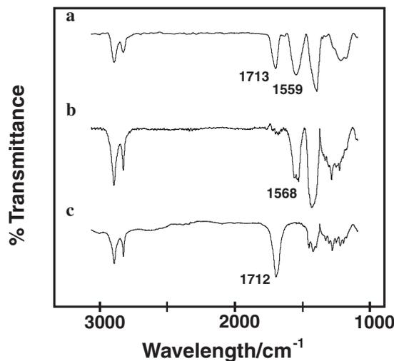
Fig. 6. FT-IR spectra attained from Au/HS( $\text{CH}_2$ ) $_{10}$ COOH colloids at pH (a) 6, (b) 11, and (c) 3.
