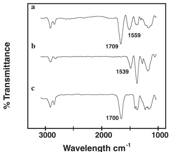
Fig. 7. FT-IR spectra attained from Au/EtSS(CH<sub>2</sub>)<sub>10</sub>COOH colloids at pH (a) 6, (b) 11, and (c) 3.
