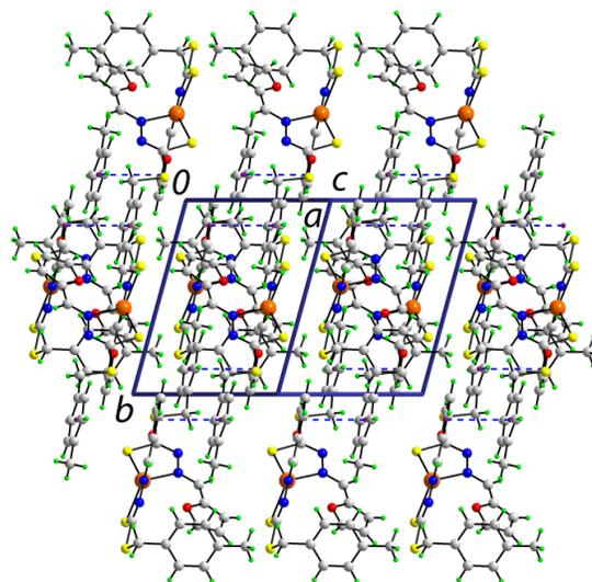
**Figure 5.** A view of the unit cell contents of **3**. The  $\pi \dots \pi$  interactions are shown as blue dashed lines.
