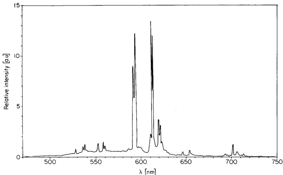
Fig. 2. The fluorescence spectra of  $\{(\text{C}_4\text{H}_9)_4\text{N}\}_3\text{Eu}(\text{NCS})_6$  crystals at 15 K.:
