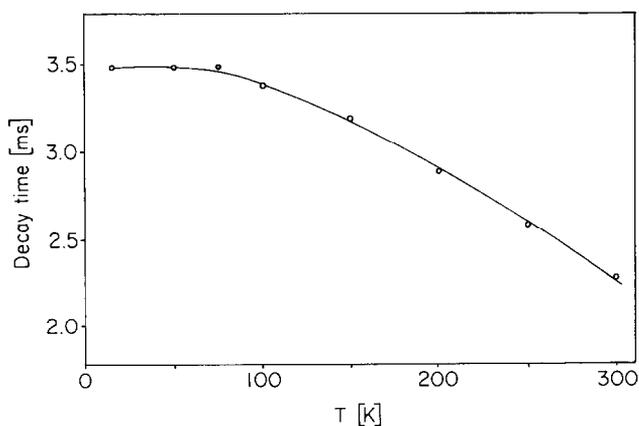
Fig. 3. The temperature dependence of fluorescence decay time of  $^5D_0$  fluorescence of  $\{(C_4H_9)_4N\}_3Eu(NCS)_6$ .
