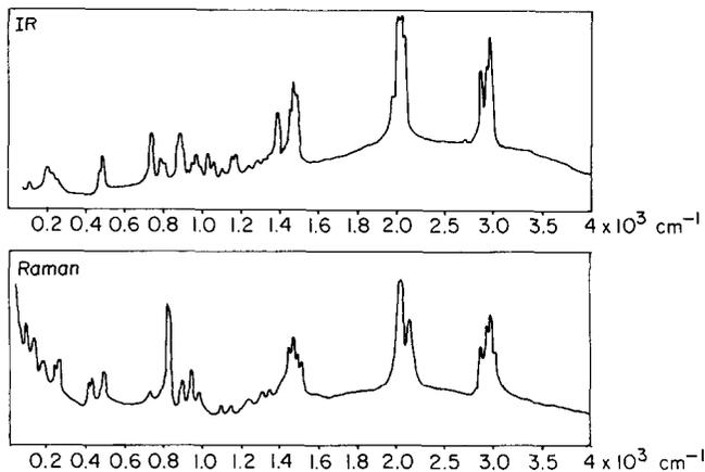
Fig. 1. The IR and Raman spectra of  $\{(\text{C}_4\text{H}_9)_4\text{N}\}_3\text{Eu}(\text{NCS})_6$  crystals.
