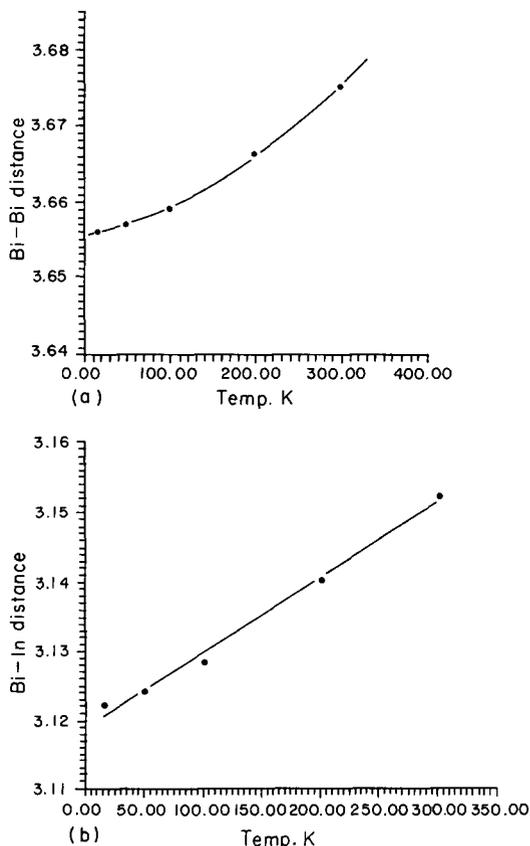
Fig. 3. Dependence of In-Bi and Bi-Bi distances on temperature.
