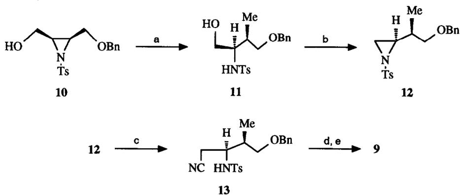
**Scheme 2.** Bn=CH<sub>2</sub>C<sub>6</sub>H<sub>5</sub>; Ts=paratoluenesulfonyl. (a) AlMe<sub>3</sub>, toluene, 75°C, 92% (see ref. 7); (b) DEAD, PPh<sub>3</sub>, THF, RT, 80%; (c) KCN, MeOH, 40°C, 82%; (d) 2M NaOH.aq., reflux, 98%; (f) see step (g) in Scheme 1.
