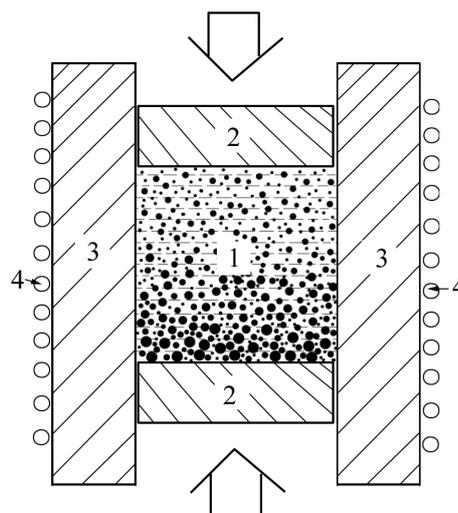
Fig. 9. Schematic structure of the hot-press autoclave. 1: benzene + BN nanoparticles; 2: piston; 3: cylinder; 4: heating coil.
