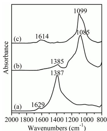
Fig. 6. FTIR absorption spectra of samples prepared at different pressures. (a) Starting material; (b) 280 °C, 50 MPa, 6 h; (c) 280 °C, 120 MPa, 6 h.
