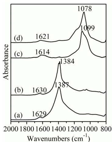
Fig. 3. FTIR absorption spectra of BN samples. (a) The starting material; (b) 240 °C, 120 MPa, 6 h; (c) 280 °C, 120 MPa, 6 h; (d) 300 °C, 120 MPa, 6 h.
