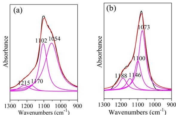
Fig. 4. Fitting results of the FTIR bands of BN samples. (a) The fitting result of the band in Fig. 3(c); (b) the fitting result of the band in Fig. 3(d). The peaks at 1054–1073  $\text{cm}^{-1}$  are attributed to *c*-BN, and those at 1100–1102  $\text{cm}^{-1}$ , 1146–1170  $\text{cm}^{-1}$ , and 1188–1215  $\text{cm}^{-1}$  to *w*-BN. (The Origin Pro 7.0 software was used in the analysis of the bands of Fig. 3(c) and (d)).
