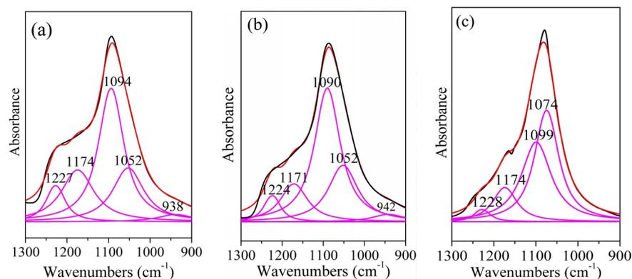
Fig. 8. Fitting results of the FTIR bands in Fig. 7. Figs. 8(a), (b) and (c) are corresponding to Figs. 7(a), (b) and (c), respectively. The peaks at 1052–1074  $\text{cm}^{-1}$  can be attributed to *c*-BN, those at 1090–1099  $\text{cm}^{-1}$ , 1171–1174  $\text{cm}^{-1}$  and 1224–1228  $\text{cm}^{-1}$  to *w*-BN.
