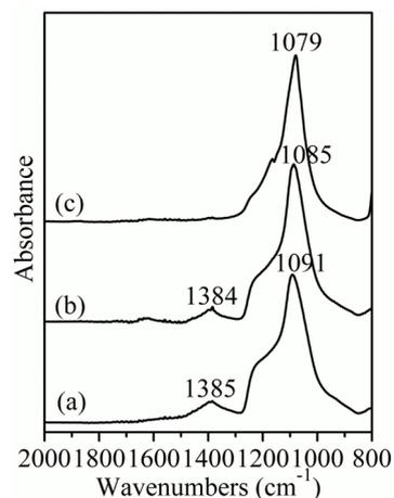
Fig. 7. FTIR absorption spectra of the samples hot-pressed for different periods of time. (a) 280 °C, 83 MPa, 1 h; (b) 280 °C, 83 MPa, 2 h; (c) 280 °C, 83 MPa, 4 h.
