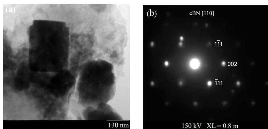
Fig. 5. TEM image and SAED pattern of *c*-BN nanocrystals. The sample was prepared by hot-pressing the starting material at 300 °C and 120 MPa, the spots in (b) can be indexed to the (1  $\bar{1}$  1), (002) and ( $\bar{1}$  11) diffractions of *c*-BN.
