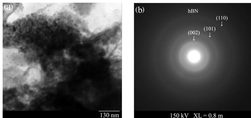
Fig. 1. TEM image and SAED pattern of the starting material. (a) coagulated *h*-BN nanoparticles, (b) the corresponding SAED pattern.
