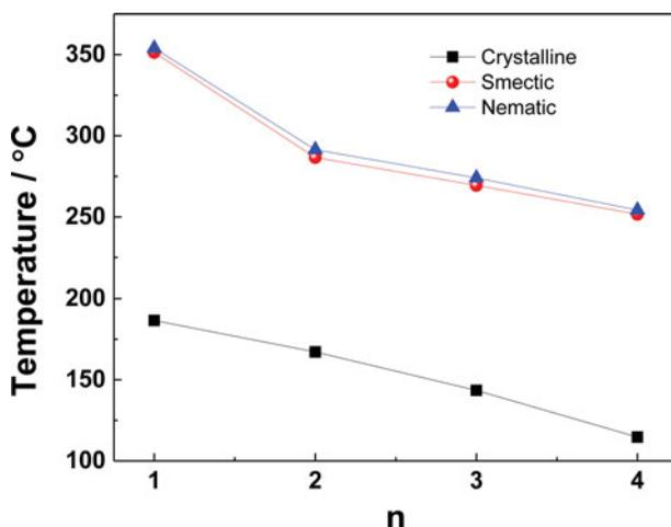
**Figure 2.** Dependence of transition temperatures of HBPE- $n$  on the length ( $n$ ) of central flexible spacer on heating run.
