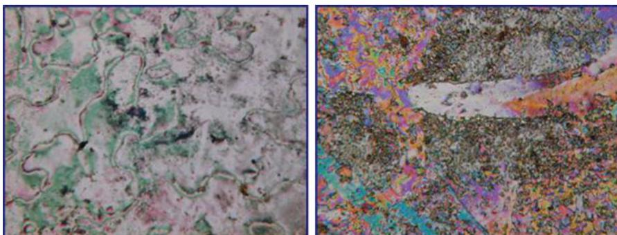
**Figure 3.** Optical photomicrographs of HBPE-4 on cooling ( $10^{\circ}\text{C}/\text{min}$ ,  $\times 100$ ): (a) nematic ( $240^{\circ}\text{C}$ ) and (b) smectic C ( $95^{\circ}\text{C}$ ).
