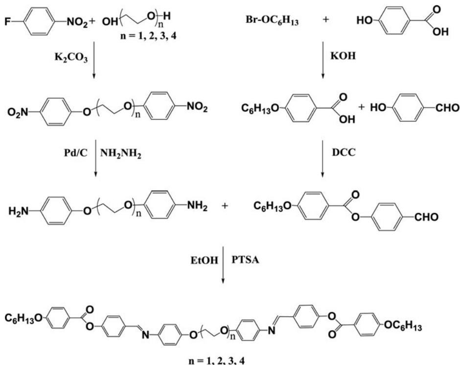
**Scheme 2.** Preparation method of HBPE-*n* series of dimers.
