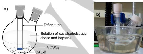
**Scheme 4.** a) Schematic representation of DKR reaction setup with compartmentalization of the catalysts; b) DKR reaction: tube with VOSO<sub>4</sub> in contact with the reaction media containing the substrate (a racemic *sec*-alcohol), vinyl decanoate (acyl donor), immobilized CAL-B and heptane.
