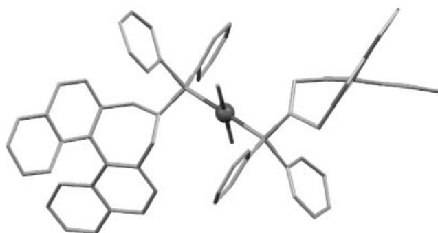
Figure 1. X-ray structure of compound **6** showing the *trans* configuration of the complex. Important bond lengths [Å] and angles [°]: P(1)–Pt 2.304(6); P(2)–Pt 2.328(4); Pt–Cl(1) 2.292(4); Pt–Cl(2) 2.305(5); P(1)–N(1) 1.690(16); P(2)–N(2) 1.727(18); P(1)–Pt–P(2) 178.9(3)°.
