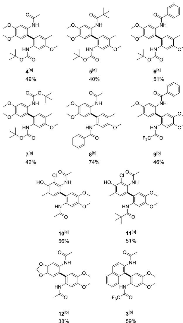
**Figure 3.** Scope of protected nonsymmetric 2,2'-diaminobiaryls. Yields of isolated products are given. [a] Electrolysis conditions: 50 °C, constant current ( $j = 5.2 \text{ mA cm}^{-2}$ ), glassy carbon anode, glassy carbon cathode, undivided beaker-type cell,  $Q = 2 \text{ F}$  (aniline **A**), solvent: HFIP/MeOH (18% v/v), supporting electrolyte: 0.09 M  $\text{Bu}_3\text{NMeO}_3\text{SOMe}$ , **A/B** = 1:2. [b] Electrolysis conditions as in [a], solvent: HFIP.
