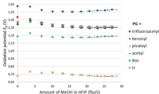
**Figure 2.** Changes in the oxidation potentials of various protected 3,4-dimethoxyanilines with increasing MeOH concentration in HFIP. WE: glassy carbon electrode tip, 2 mm diameter; CE: glassy carbon rod; RE: Ag/AgCl in saturated LiCl/EtOH; solvent: HFIP with 0–27% v/v MeOH; supporting electrolyte: 0.09 M  $\text{Bu}_3\text{NMeO}_3\text{SOMe}$ .
