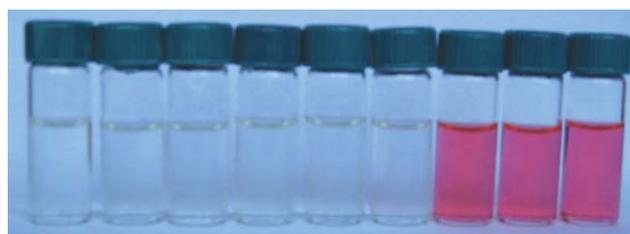
**Fig. 3** The color change of **2** in pH 7.40 of phosphate buffer solution (MeOH–H<sub>2</sub>O = 3:7, v/v) in the presence of 10 equiv. of certain amino acids. From left to right: none, Tyr, Glu, Met, Lys, His, Cys, Hcy and GSH. [**2**] =  $2.0 \times 10^{-5}$  M.
