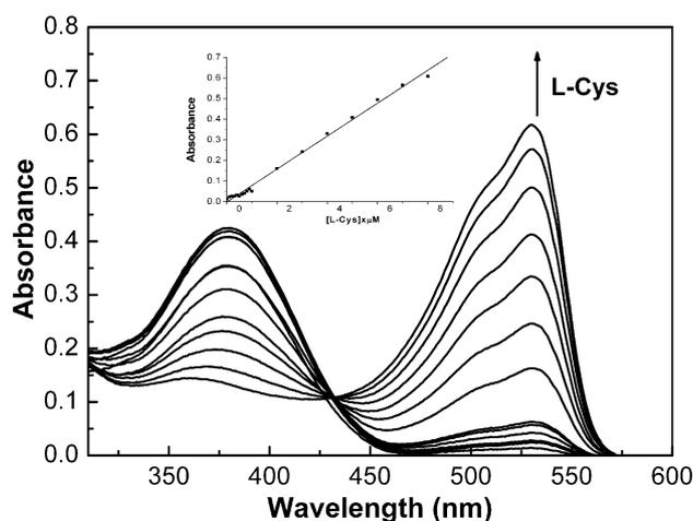
**Fig. 1** UV-Vis spectra of **2** in pH 7.40 of phosphate buffer solution (MeOH–H<sub>2</sub>O = 3:7, v/v) in the presence of Cys. Inset: plot of absorbance at 530 nm vs. concentration of Cys. [**2**] =  $2.0 \times 10^{-5}$  M. [Cys] = 0, 0.1, 0.2, 0.3, 0.4, 0.5, 0.6, 0.7, 0.8, 0.9, 1.0, 2.0, 3.0, 4.0, 5.0, 6.0, 7.0 and 8.0  $\mu$ M, respectively.
