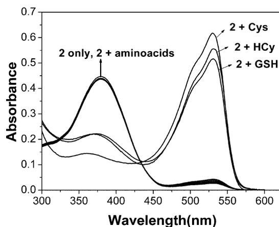
**Fig. 2** Absorbance spectra of **2** in pH 7.40 of phosphate buffer solution (MeOH–H<sub>2</sub>O = 3:7, v/v) in the presence of 0.8 equiv. of Cys, 0.4 equiv. of Cys, GSH and other amino acids. Amino acids containing: Gly, Ser, Asp, Met, Asn, Lys, Tyr, Trp, Arg, and His. [**2**] =  $2.0 \times 10^{-5}$  M.
