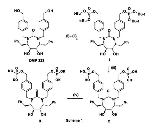
(i) (Et)<sub>2</sub>NP(OBu-t)<sub>2</sub>/tetrazole/THF/0 °C (5 min); 23 °C (15 min) (ii) m-chloroperbenzoic acid/-40 °C (5 min); 23 °C (15 min) (iii) Amberlyst 15/CH<sub>3</sub>OH/reflux/5 h (iv) 4 equiv KHCO<sub>3</sub>/THF/23 °C
