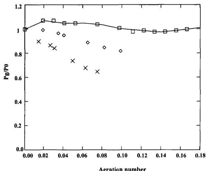
**Figure 6.** Values of  $P_g/P_O$ . The boxes correspond to the values obtained by Saito et al. (1992) for the SRGT turbine. The solid curve is the spline of interpolation of these data which is used when deriving the data for the secondary SHP impellers. The diamonds are the data as observed for the entire stirrer in Stavanger. The crosses are the data derived, as described in the text, for the secondary SHP impellers.
