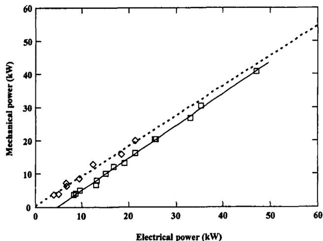
**Figure 2.** Mechanical power as a function of electrical power. The boxes are the data from the Stavanger bioreactor. The diamonds are the data from Strängnäs. The solid and dash lines are the fits to the Stavanger and Strängnäs data according to Equation (5) with the parameters given in the text.
