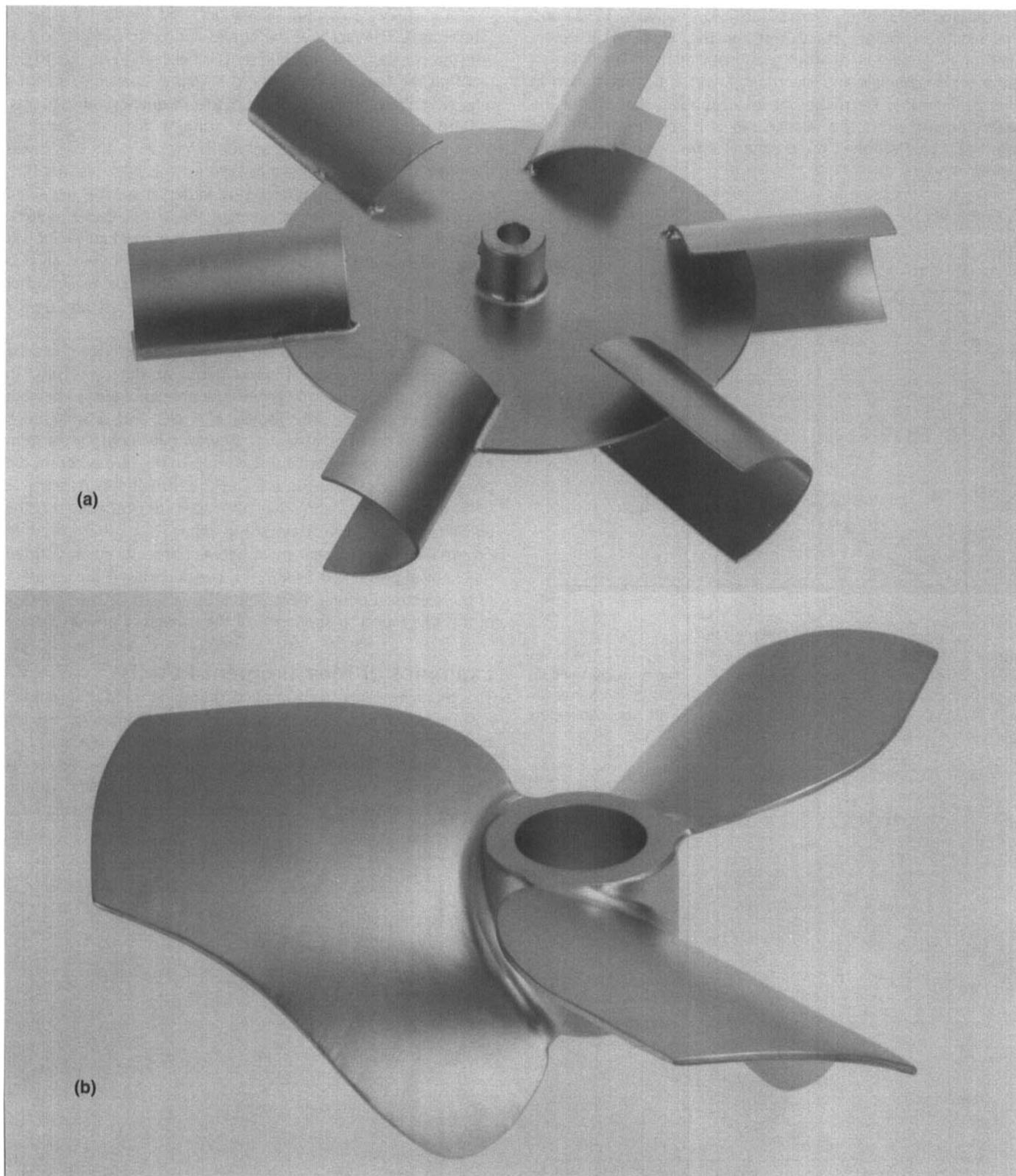
Figure 5. Models of the SCABA 6SRGT turbine (a) and the three blade SHP1 hydrofoil type impeller (b) employed at Strängnäs.
