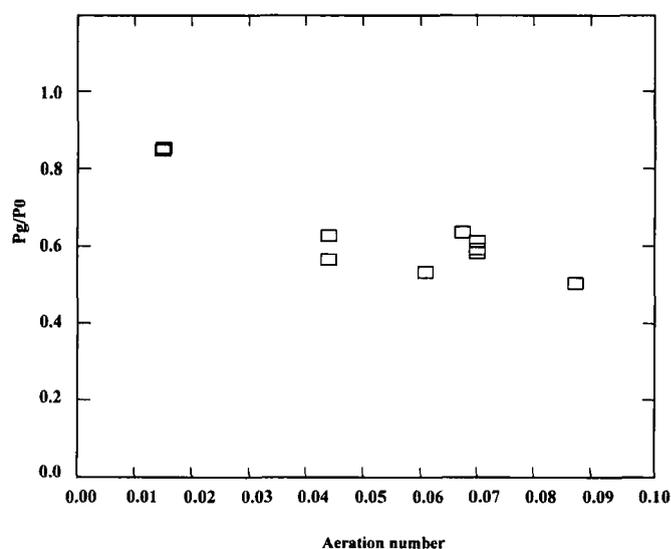
**Figure 4.** Ratio of aerated to unaerated power as a function of the aeration number when using three Rushton turbines in the Strängnäs bioreactor. The data are from a fermentation operation where both air flow and agitator speed have been varied.
