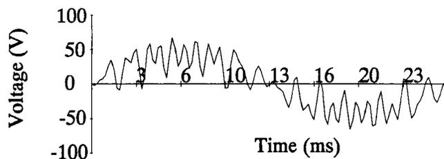
Figure 1. Typical voltage signal produced by a Danfoss VLT100-150 speed control unit.
