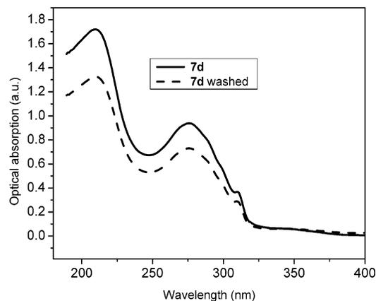
**Figure 6.** UV absorbance spectra of **7d** after thermal curing (1 h, 150 °C) and after curing and solvent rinsing (THF).
