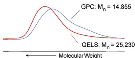
**Figure 2.** Comparison of GPC and quasi-elastic light scattering (QELS) results on molecular-weight determination of polymer **5b**. GPC underestimates the  $M_n$  value by a factor of 1.6–1.8.
