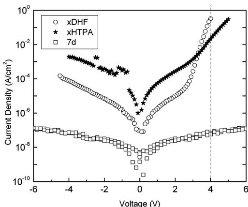
**Figure 8.** Comparison of the electrical properties of devices based on different polymer films for ITO/polymer/Al structure.
