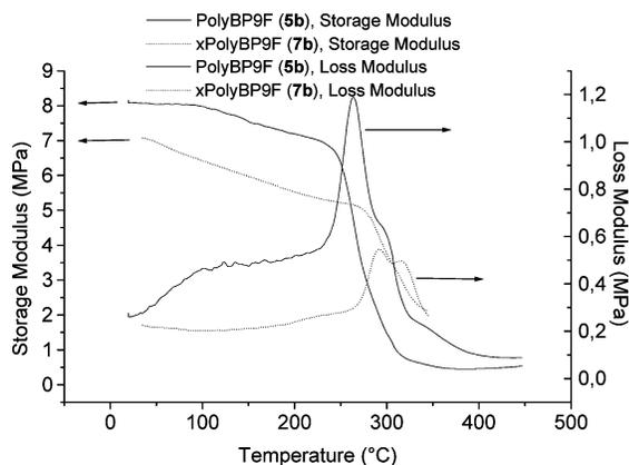
**Figure 3.** Dynamic mechanical analysis (DMA). Storage and Loss Modulus for **5b** (—) and **7b** (···).
