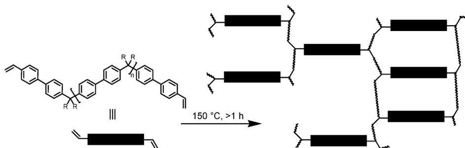
**Figure 5.** Schematic representation of the formation of a cross-linked film.
