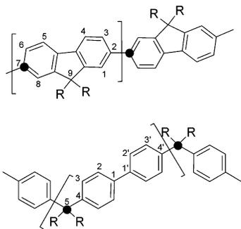
**Figure 1.** Structural comparison of polyfluorene (above; repeating unit length: 8.4 Å, ●↔●) and poly(biphenylmethylene) (below; repeating unit length: 10.3 Å, ●↔●).
