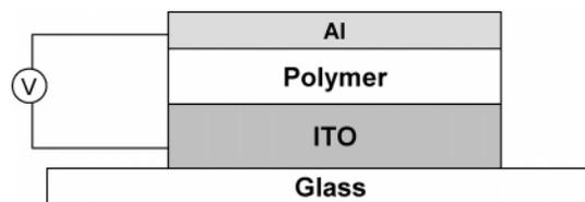
**Figure 7.** Device structure of the fabricated devices.
