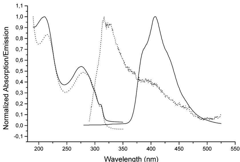
**Figure 4.** Absorption and photoluminescence spectra of polymers **5d** (···) and **7d** (—).
