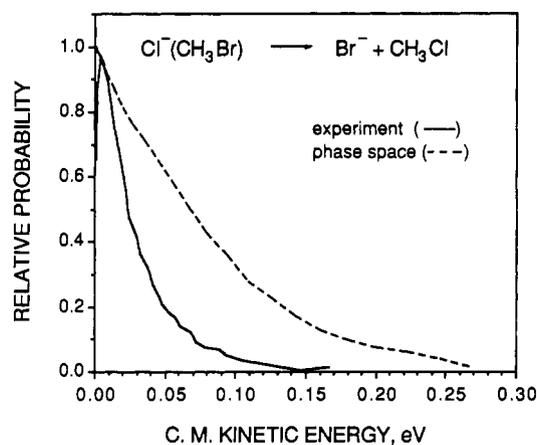
**Figure 2.** Experimental and theoretical kinetic energy release distributions for the metastable displacement reaction of  $\text{Cl}^-(\text{CH}_3\text{Br})$ . The theoretical curve is calculated for  $\text{Cl}^-(\text{CH}_3\text{Br})$  complexes with internal energies between 0.4 and 0.5 eV (see text).
