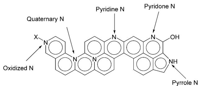
**Scheme 2.** Possible structures of nitrogen doped to carbon.
