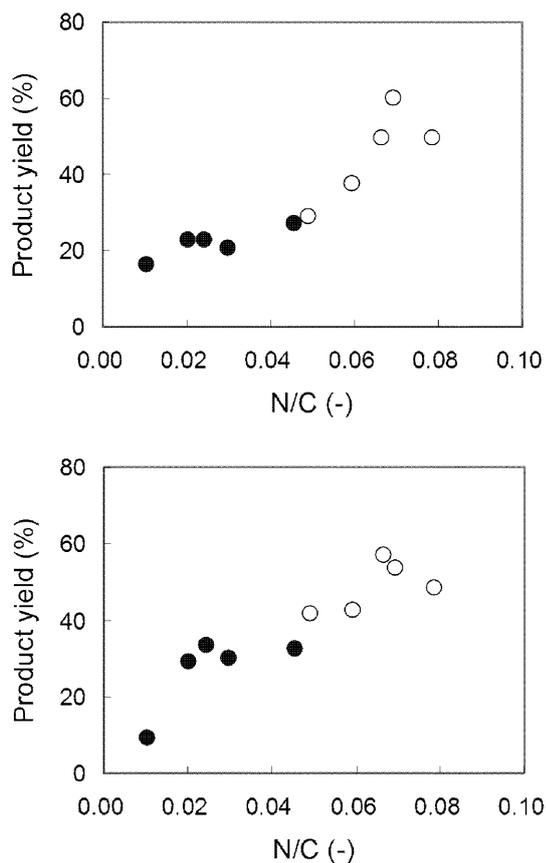
**Figure 4.** Plot of the product yield in (*top*) Knoevenagel condensation and (*bottom*) transesterification reaction against the N content for nitrogen-doped AC- (open circle) and CB-derived (closed circle) carbon catalysts.
