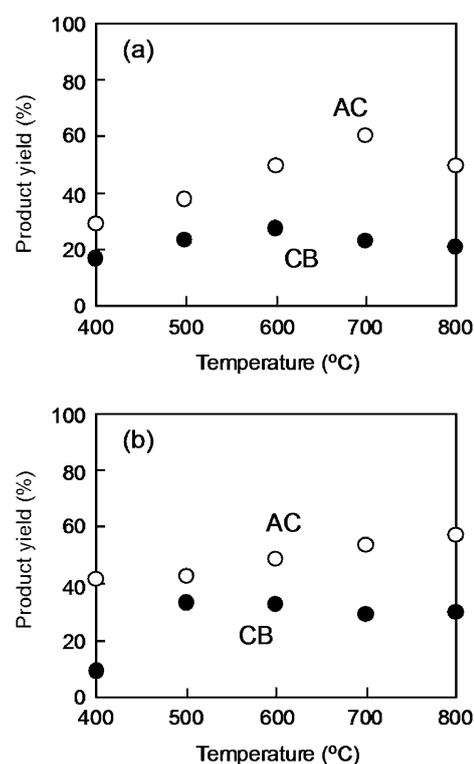
**Figure 1.** Results of (a) Knoevenagel condensation and (b) transesterification reaction using nitrogen-doped AC- and CB-derived carbon catalysts prepared *via* ammoxidation at different temperatures (NH<sub>3</sub> concentration 90%, ammoxidation time 1 h).
