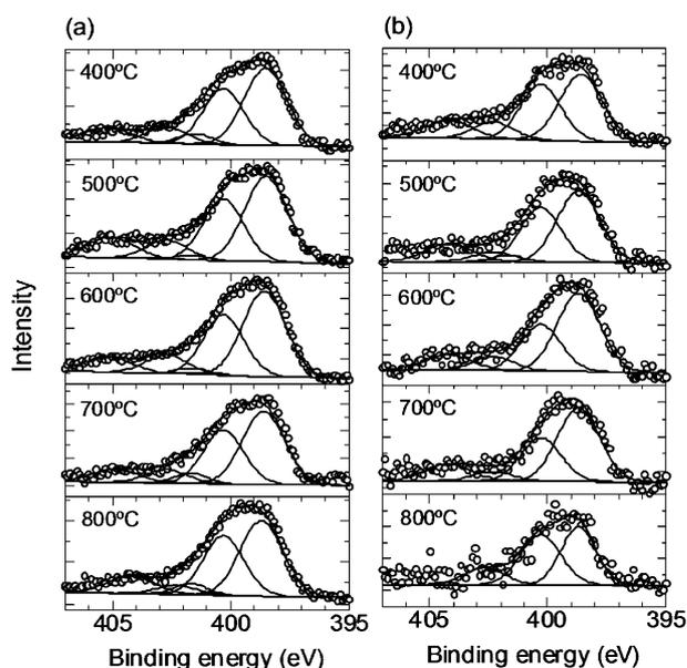
**Figure 3.** XPS spectra of AC- (a) and CB- (b)-based catalysts prepared by ammoxidation with 90% NH<sub>3</sub> for 1 h at the different temperatures given.
