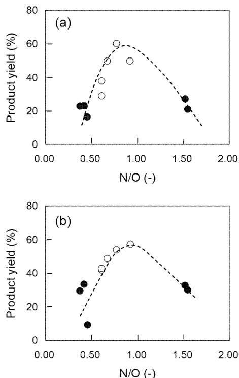
**Figure 6.** Plots of the product yield in Knoevenagel condensation (a) and transesterification reaction (b) against the N/O ratio for the AC- (open circles) and CB- (closed circles) derived nitrogen-doped carbon catalysts
