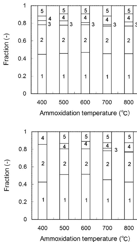
**Figure 5.** Distributions of N species of (*top*) AC- and (*bottom*) CB-derived carbon catalysts prepared by ammoxidation with 90%  $\text{NH}_3$  at the different temperatures given. 1 = pyridine-type; 2 = pyrrole/pyridone-type; 3 = quaternary-type; 4 = oxidized-type; 5 = adsorbed  $\text{NO}_x$ .
