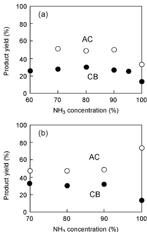
**Figure 2.** Results of (a) Knoevenagel condensation and (b) transesterification reaction using nitrogen-doped AC- and CB-derived carbon catalysts prepared *via* ammoxidation with different  $\text{NH}_3$  concentrations (ammoxidation temperature  $600^\circ\text{C}$ , time 1 h).
